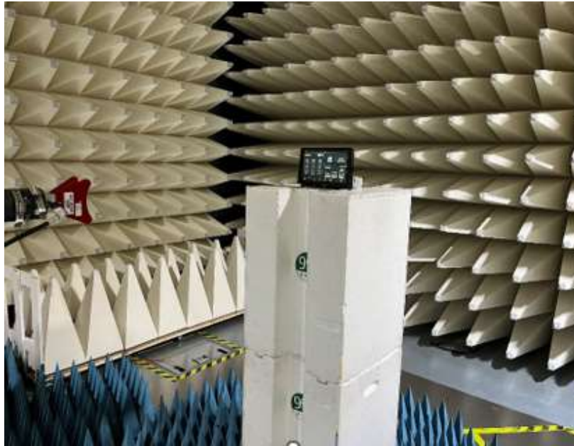
Figure C7. High Range Radiated Emission test setup 18-26GHz
