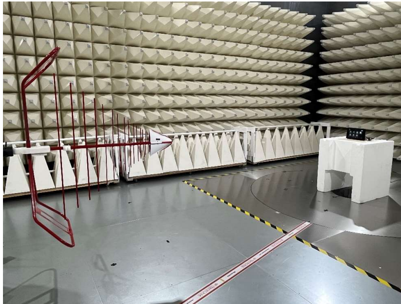
Figure C5. Low Range Radiated Emission test setup
