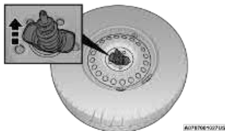
Reinstalling The Retainer
