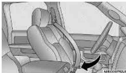
Inserting Latch Plate Into Buckle
