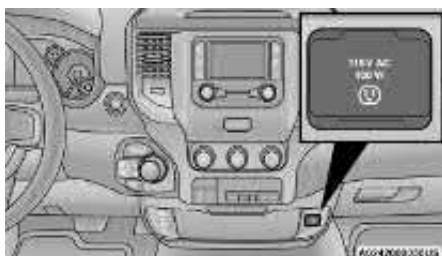
Center Stack Power Inverter
