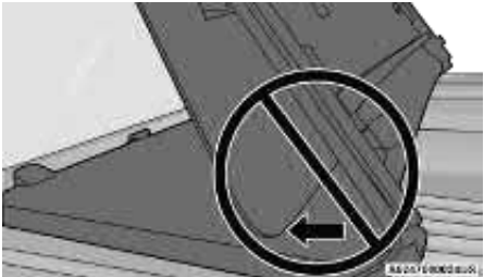
Incorrect Folding – Will Cause Damage
