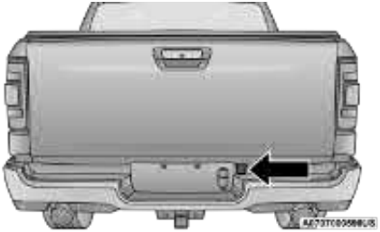
Access Hole Cover Location
