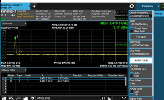
Hopping enabled Low Channel 2307MHz-2407MHz
