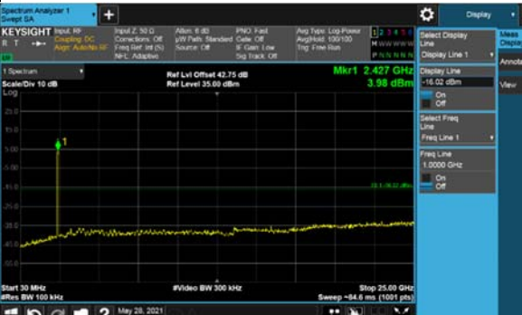
Hopping enabled 30 MHz-25 GHz
