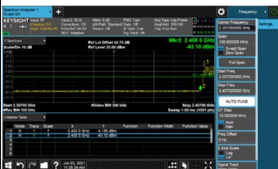
Hopping enabled High Channel 2473MHz-2573MHz
