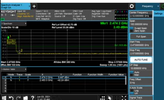
Hopping enabled High Channel 2473MHz-2573MHz
