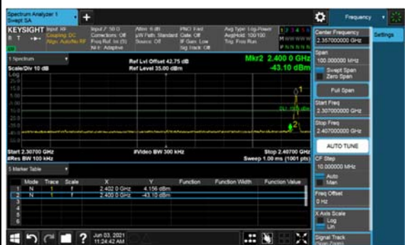
Hopping disabled High Channel 2473MHz-2573MHz
