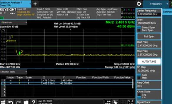
Hopping enabled_High Channel 2473MHz-2573MHz
