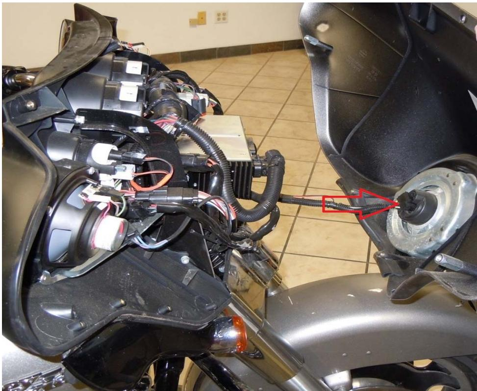
5. Mount our unit using the factory rubber isolator mounts and the torx set screw shown in the picture below
