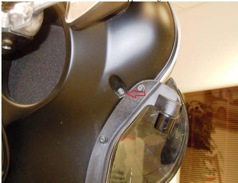
3. Locate and remove the two bolts at the bottom of the inner faring one each side
