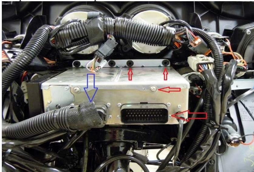
8. On the 23 Pin connector show above with a Blue arrow Connect the Red wire using the supplied t tap to pin 20 on the main radio plug Connect the Black wire using the supplied t tap to pin 19
