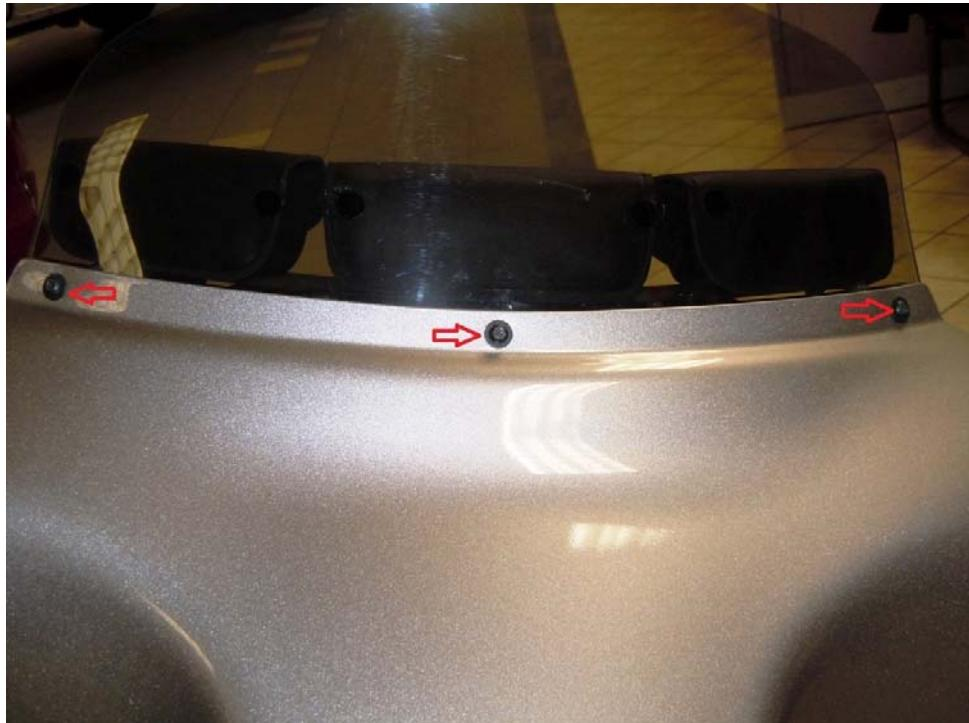
2. Locate and remove the two bolts on the upper fairing one on each side
