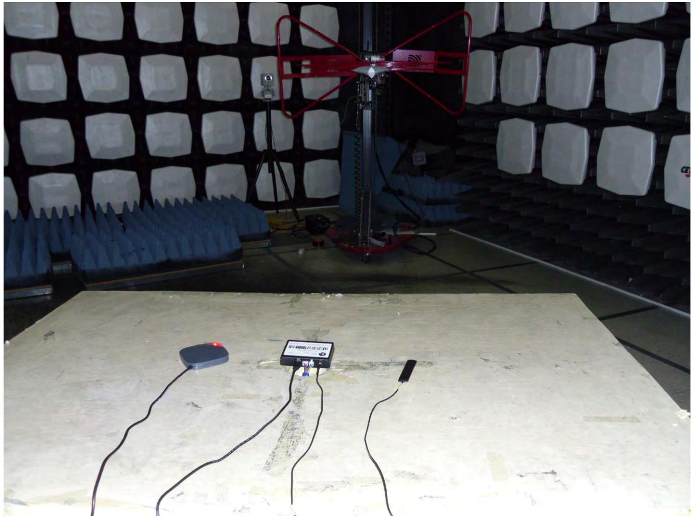
4 Radiated Emissions Above 1GHz Measurement for 47 CFR Part 15B according to ANSI C63.4
