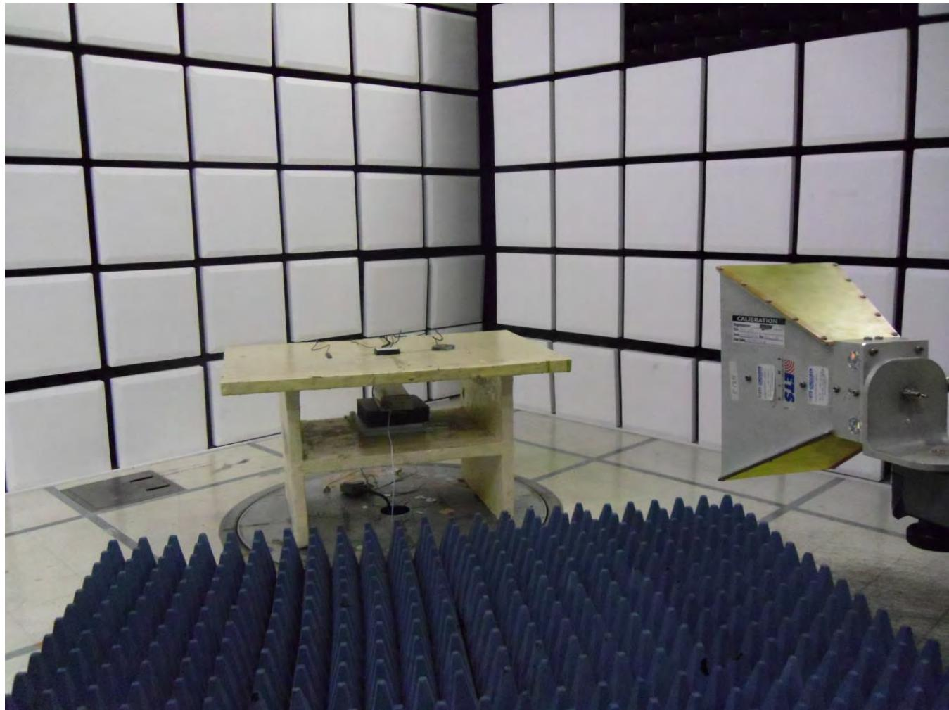
5 Radiated Emissions Above 1 GHz Measurement for 47 CFR Part 15.247, Part 22 and Part 24 as well as for RSS-247, RSS-132, RSS-133 according to ANSI C63.26
