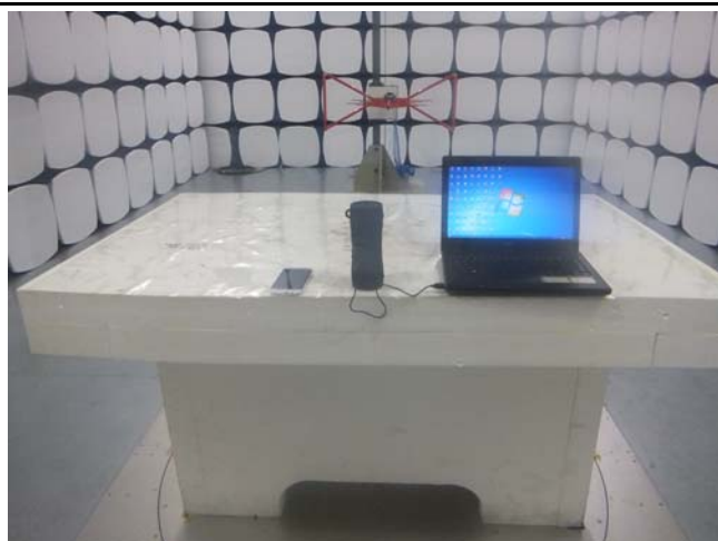
Radiated Spurious Emissions Test Setup Below 1GHz
