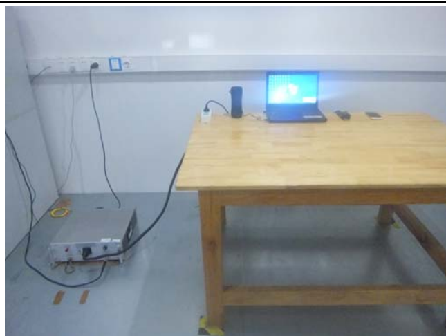
Conducted Emissions Test Setup Front View
