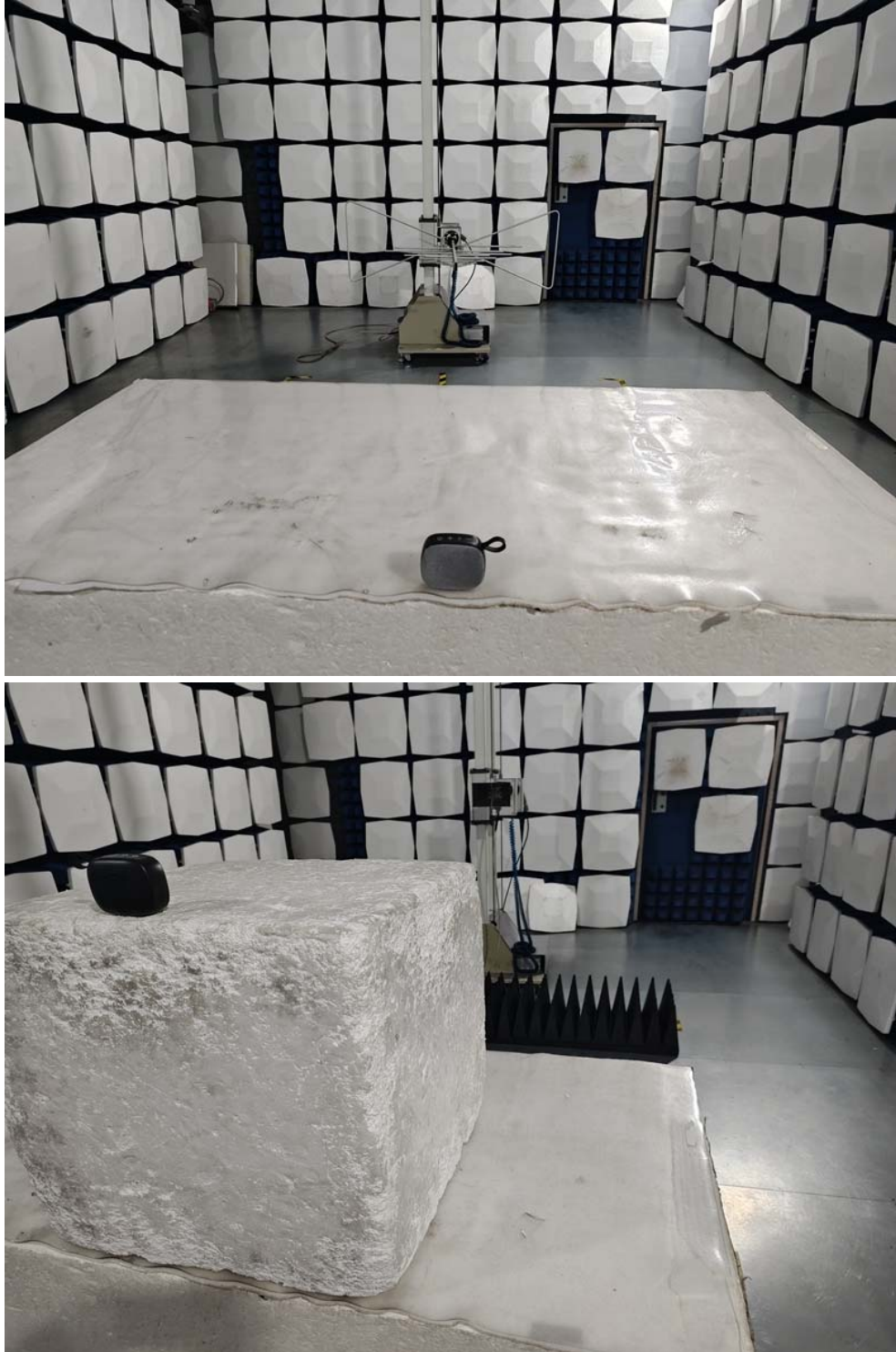
Radiated emission test view
