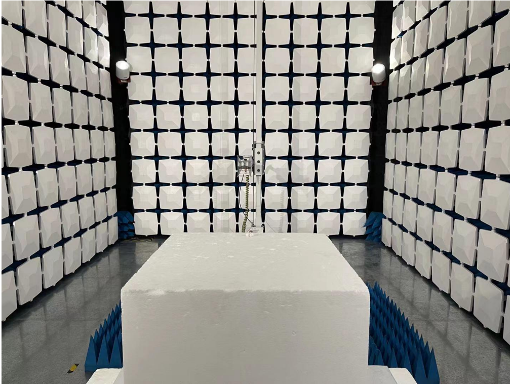
Above 1GHz for radiated emission test setup
