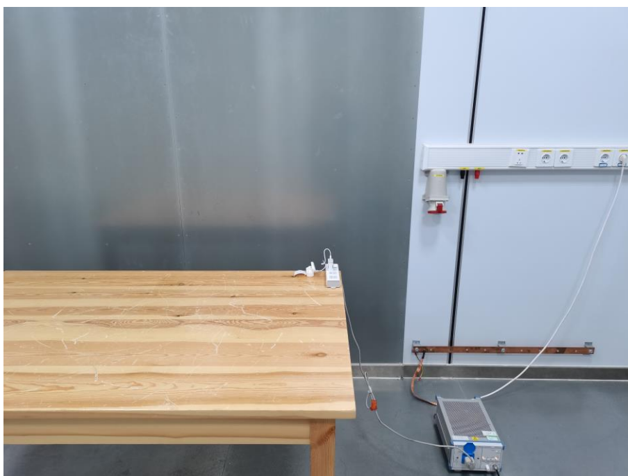
Fig. 4 Power line conducted emission setup photo
