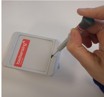
Figure 4: The Piconode can be opened making use of a 2-mm screwdriver
