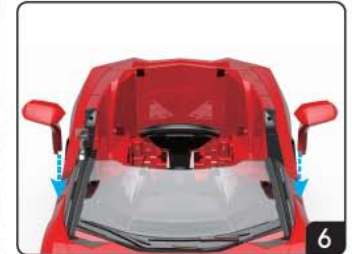
Aim the fastener of left and right mirror respectively towards the relevant socket of car body, and fix it down until it's locked.
