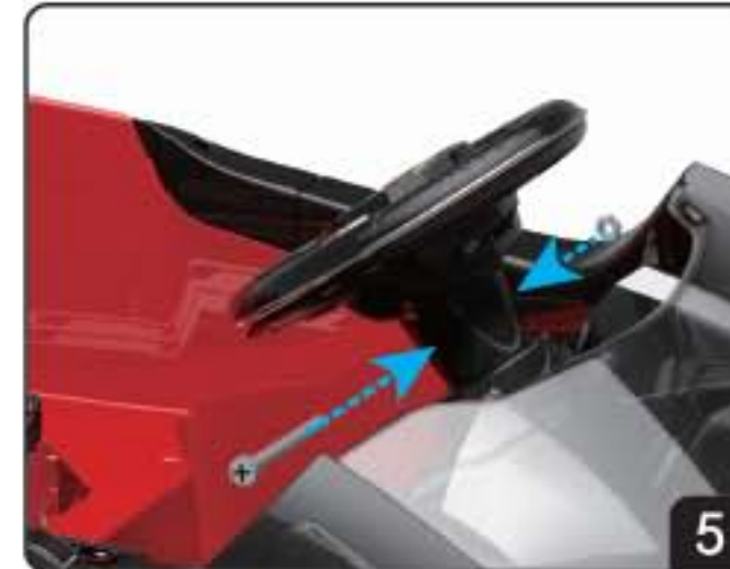
1.5 Lock the steering wheel by the screw and nut.
