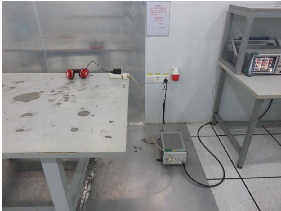
1 Photo of Power Line Conducted Emission Measurement
