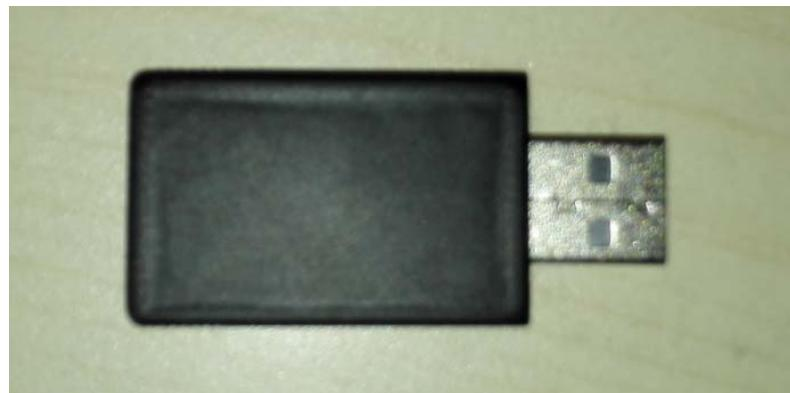
**Step 5:** Connect to your host main board with usb interface and the main board was setup in the HITACHI smart projector. BW8800 can not work alone ,it must be working with main board .
