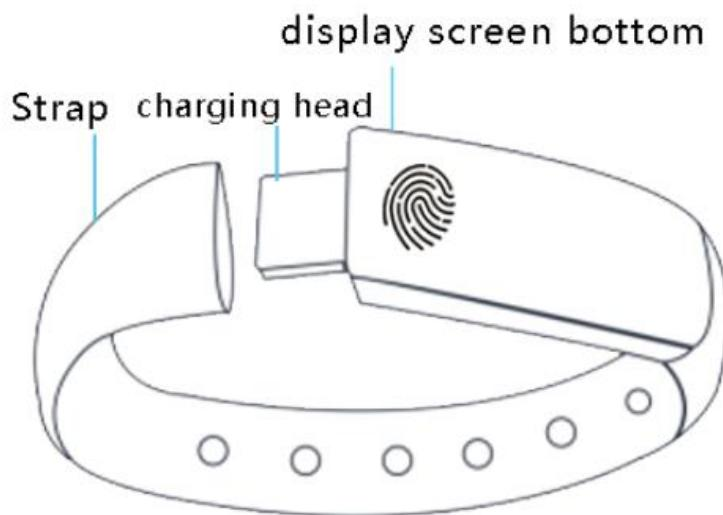
( Figure: the figure for smart bracelet USB interface to open )
