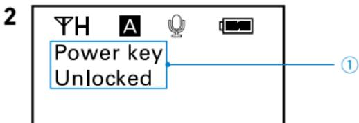
① Menu display section. Displays various functions. Press the + or - button to switch functions.
