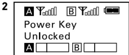
**Power key.** Long press the SET button to unlock or locked the power key. Lock the power key to prevent the receiver being turned off unwittingly while using.
