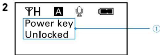
**(1) Menu display section.** Displays various functions. Press the + or - button to switch functions.
