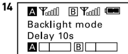
**Set backlight.** Set the background LED light to ON or Delay 60 /30 /10 seconds or OFF. Default is "Delay 10s."
