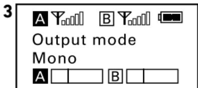
**Output mode.** The output mode can be selected to mono or stereo. When the output mode is mono, the audio from left and right channel will be mixed. When it is stereo, the left (Group B) and right (Group A) audio channel output will be separated. System default is mono.
