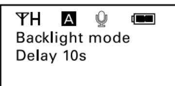
**Set Backlight.** Select ON, OFF or Delay 10 / 30 / 60 seconds. Default is "Delay 10s."
