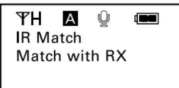
**IR Match.** Set to match with the receiver. The screen will display "Matching" when in process. After successful matching, it will indicate "Sync finished."
