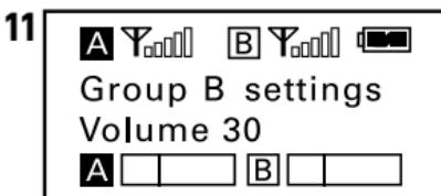
**Set output volume.** Set the volume of output audio within the range 0 to 30. The setting is retained even after the power is turned off. Default is 30.
