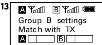
**Infrared matching function.** Match the receiver and transmitter via infrared. Details of operation, please refer to "Match the channel of receiver and transmitter" (page 24).
