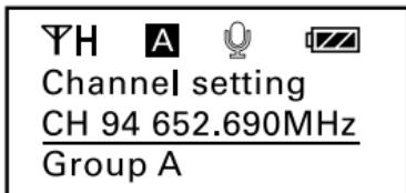
**Select Channel.** There are 96 channels with carrier frequency ranging from 614MHz to 696MHz. Default is “Channel 01” and “614.560MHz.”
