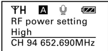
**Select RF power level.** You can set the transmitted RF power to High, Middle or Low. Default is “High.”
