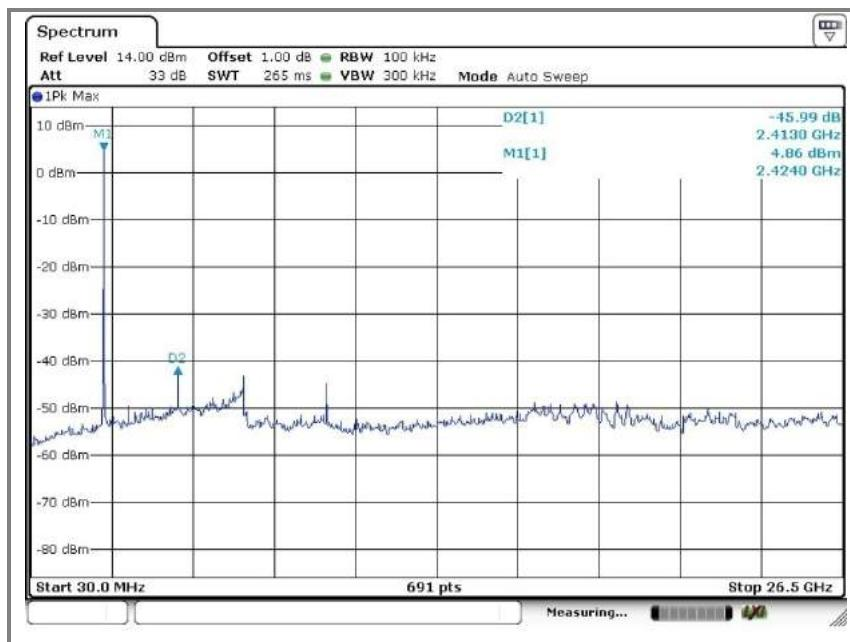
**B. Middle channel (2.437 MHz)****Reference level measurement 1**
