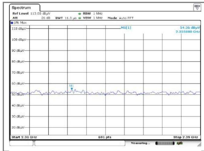
**Reference level measurement**
