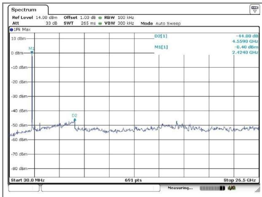
**C. High channel (2.462 MHz)****Reference level measurement 1**
