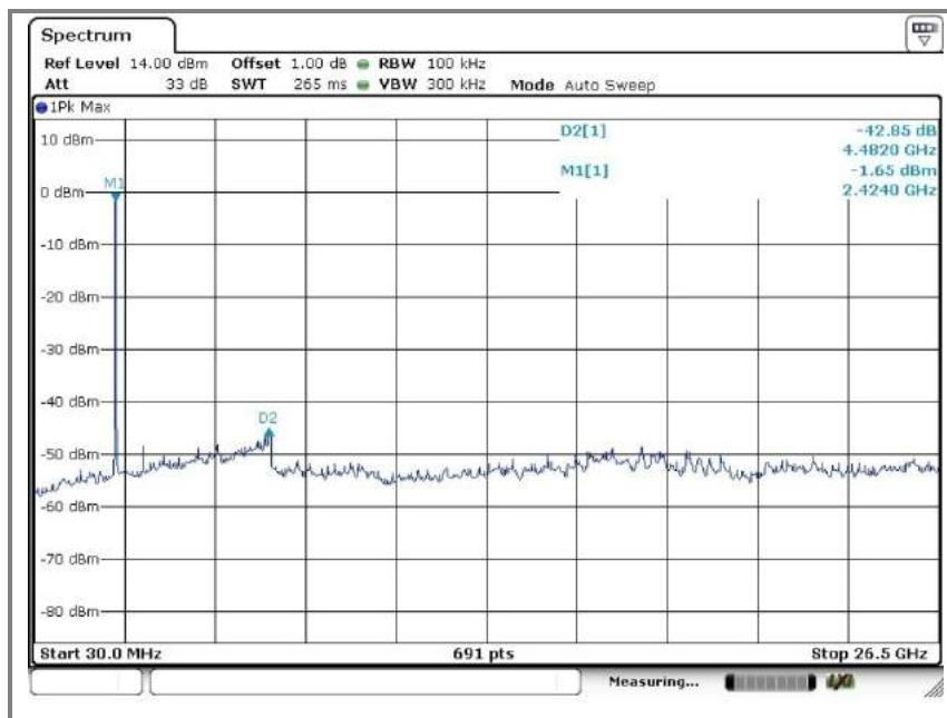
**B. Middle channel (2.437 MHz)****Reference level measurement 1**
