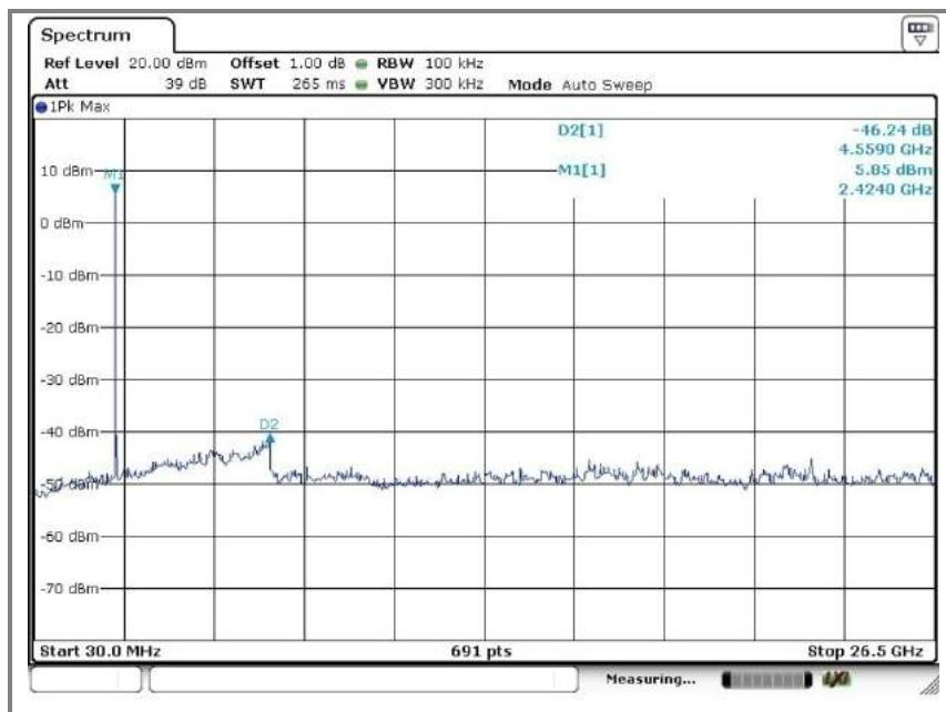
**C. High channel (2.480 MHz)****Reference level measurement 1**
