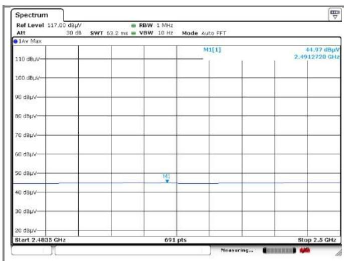
**Reference level measurement**
