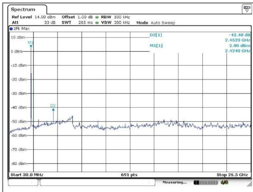
**C. High channel (2.462 MHz)****Reference level measurement 1**
