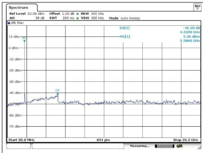
**B. Middle channel (2.440 MHz)****Reference level measurement 1**
