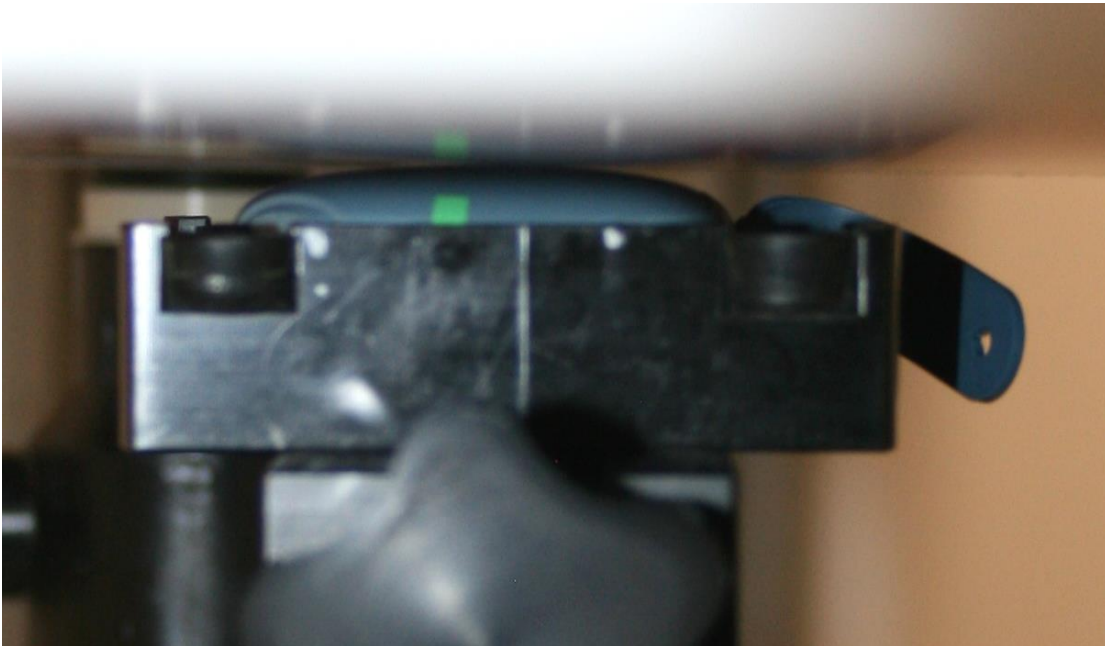
Guardian module: Front side of the device against the phantom, 0mm separation
