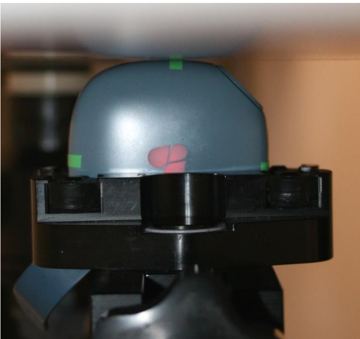
Guardian module: Bottom right side of the device against the phantom, 0mm separation
