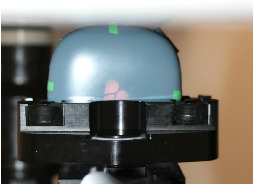
Guardian module: Top Left side of the device against the phantom, 0mm separation
