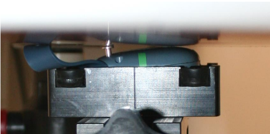
Guardian module: Back side of the device against the phantom, 0mm separation
