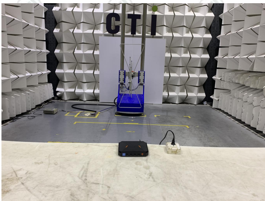
Radiated spurious emission Test Setup-2(Below 1GHz)
