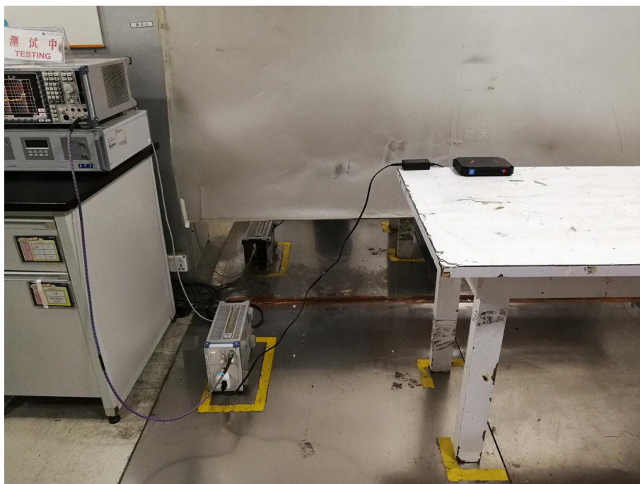
Conducted Emissions Test Setup
