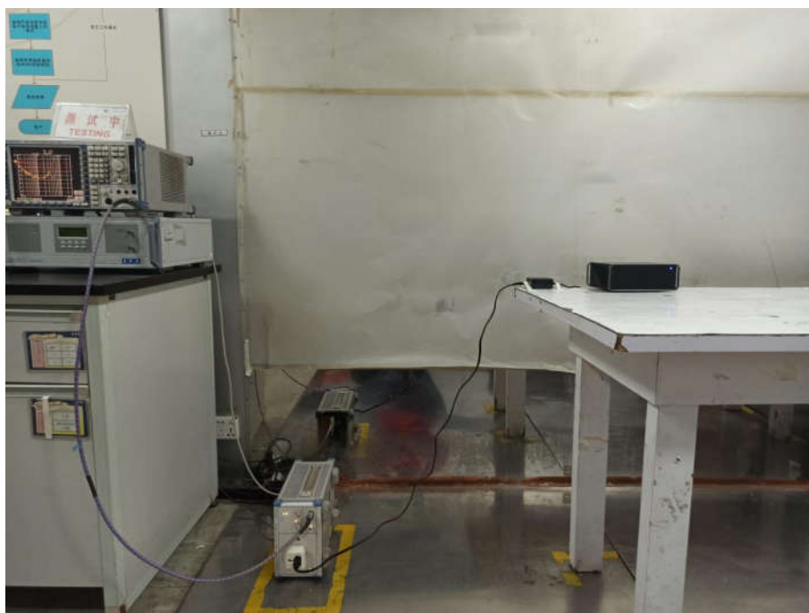
Conducted Emissions Test Setup
