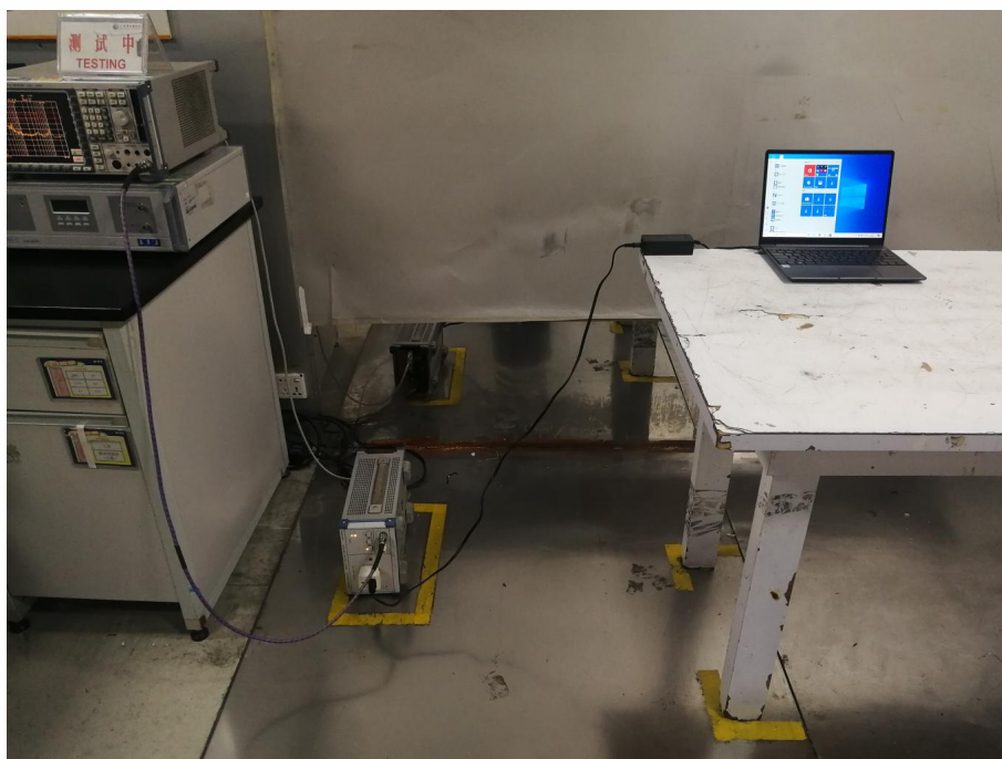
Conducted Emissions Test Setup
