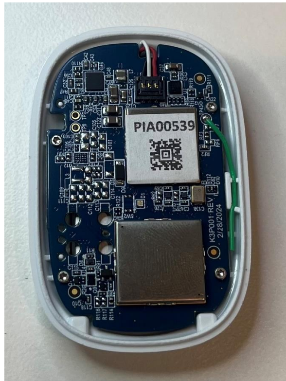
Open Pod green wire is antenna.
