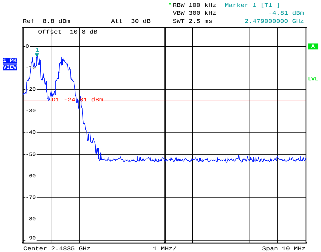
Plot 4.13 Conducted Band Edge, with GFSK (Hopping)
