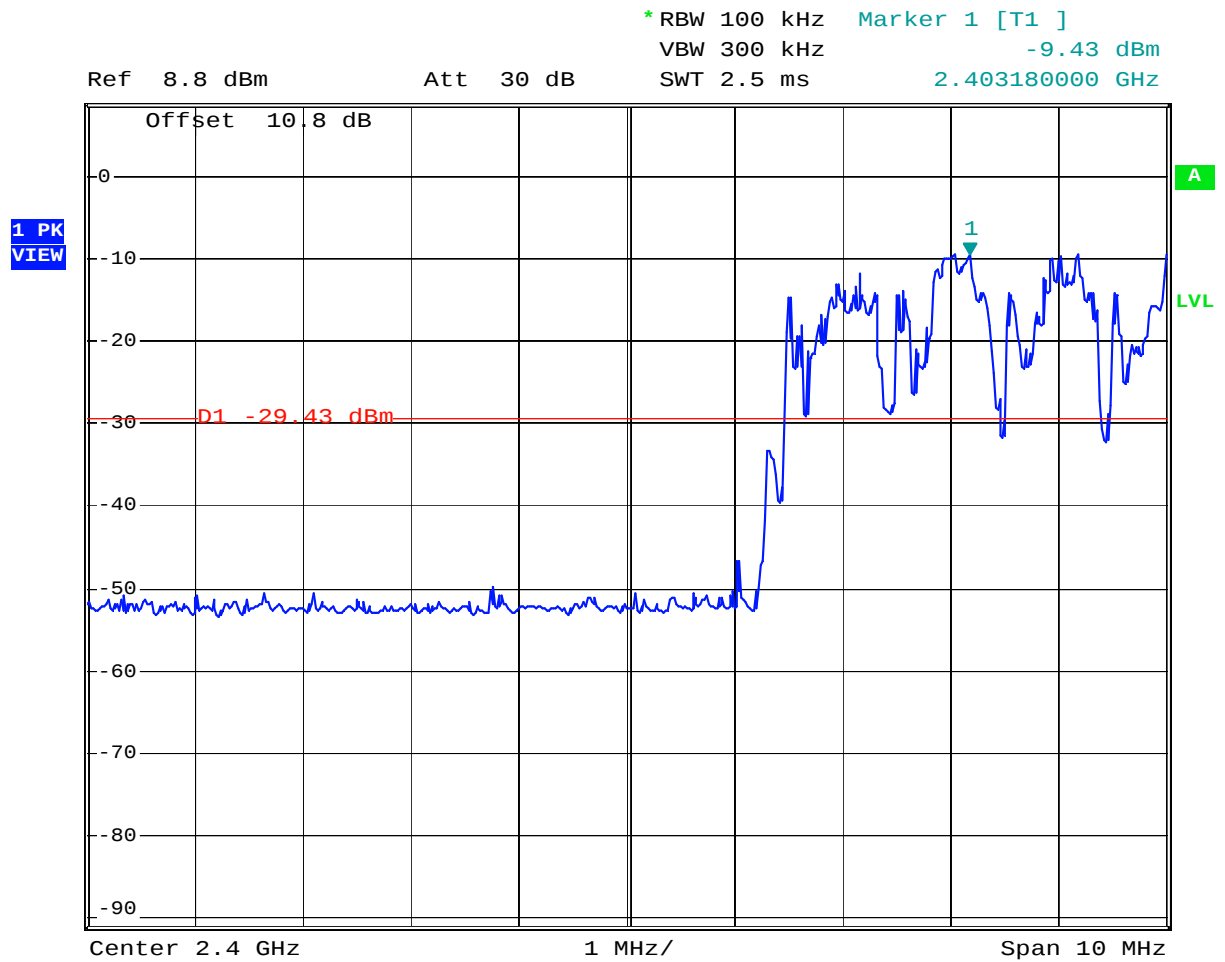
Plot 4.15 Conducted Band Edge, with \pi/4 -DQPSK (Hopping)
