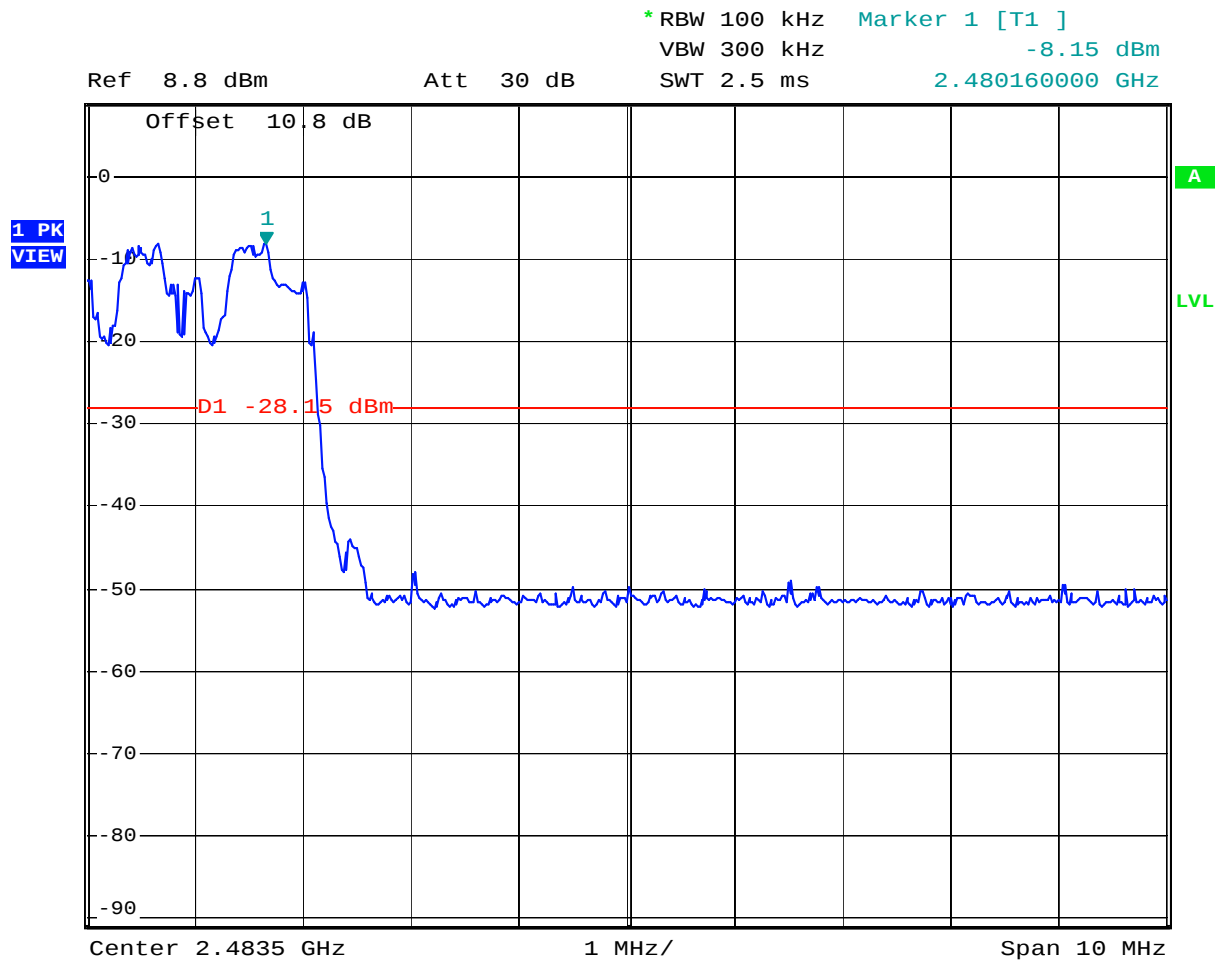
Plot 4.17 Conducted Band Edge, with \pi/4 -DQPSK (Hopping)
