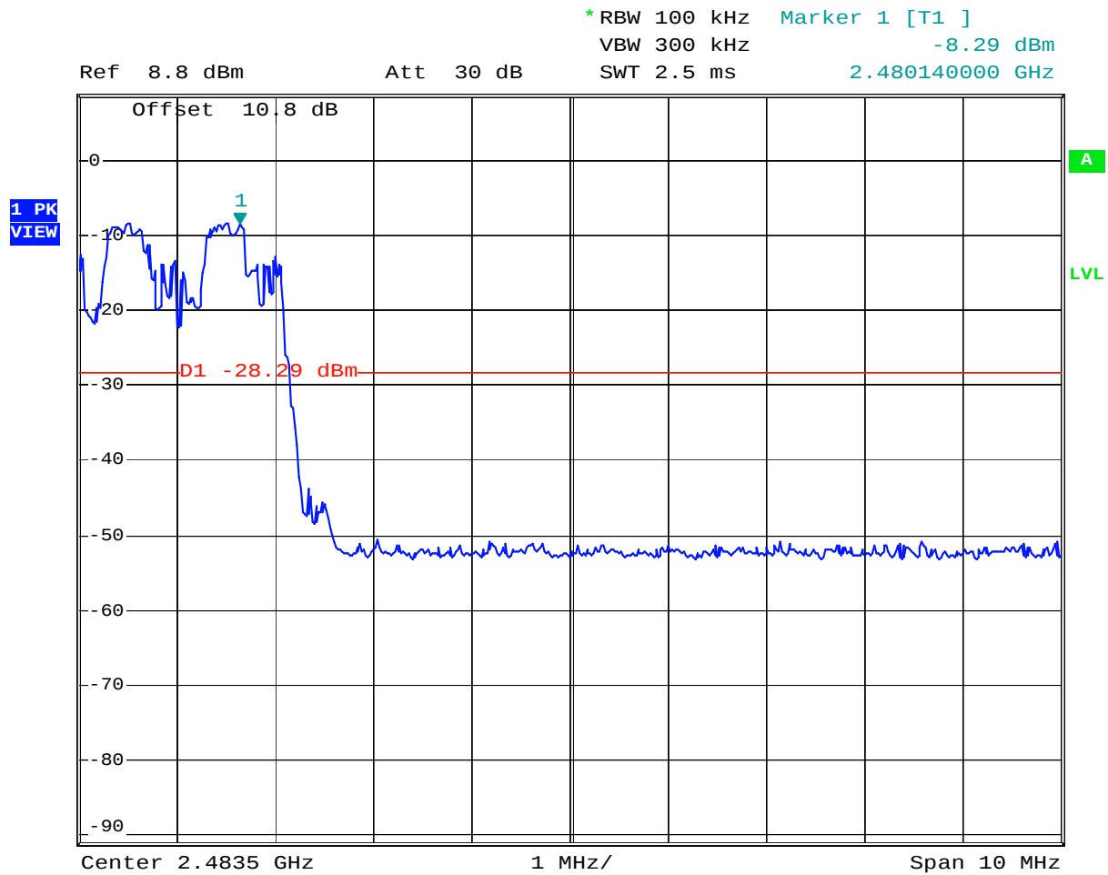
Plot 4.21 Conducted Band Edge, with 8DPSK (Hopping)
