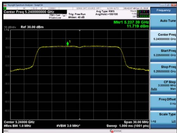
U-NII-1, 802.11ac VHT20, Channel No.: 48
