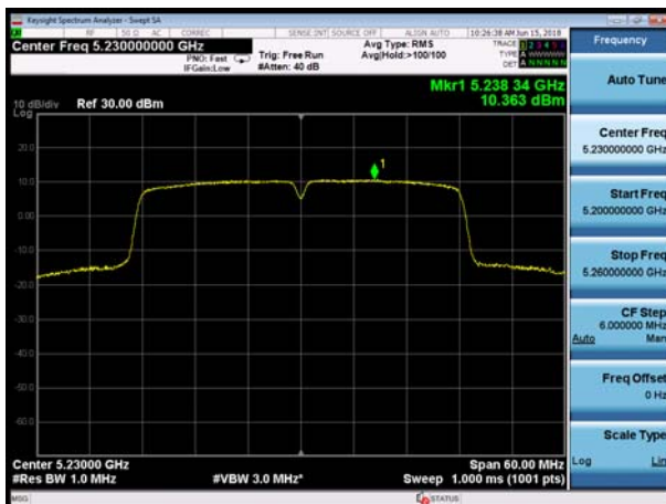
U-NII-1, 802.11ac VHT40, Channel No.: 38
