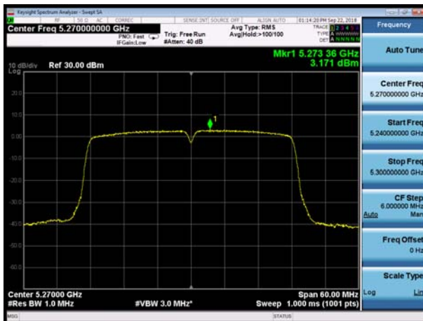
U-NII-2A, 802.11ac VHT40, Channel No.: 54
