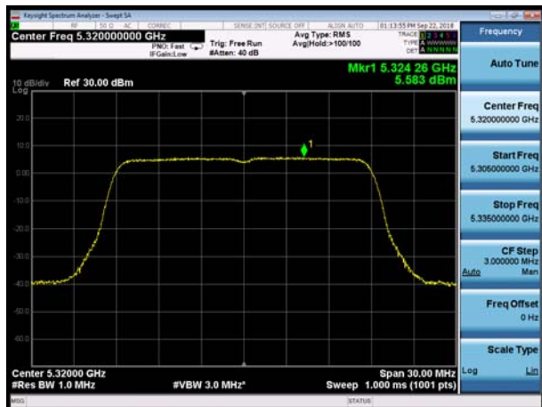
U-NII-2A, 802.11ac VHT20, Channel No.: 64
