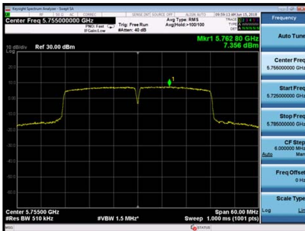
U-NII-3, 802.11ac VHT40, Channel No.: 151
