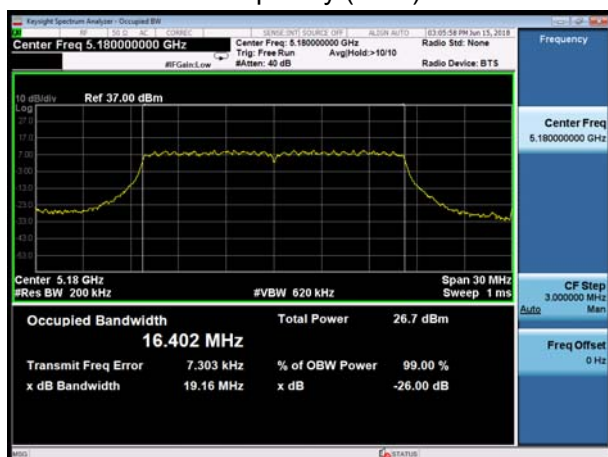
U-NII-1, 802.11a Carrier frequency (MHz): 5200
