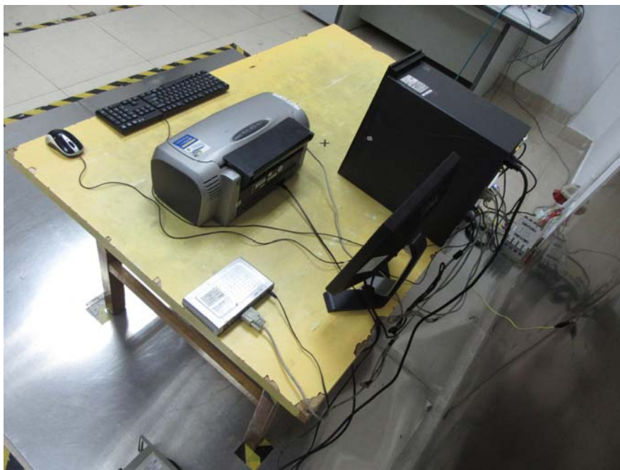
Conducted Emission Rear View
