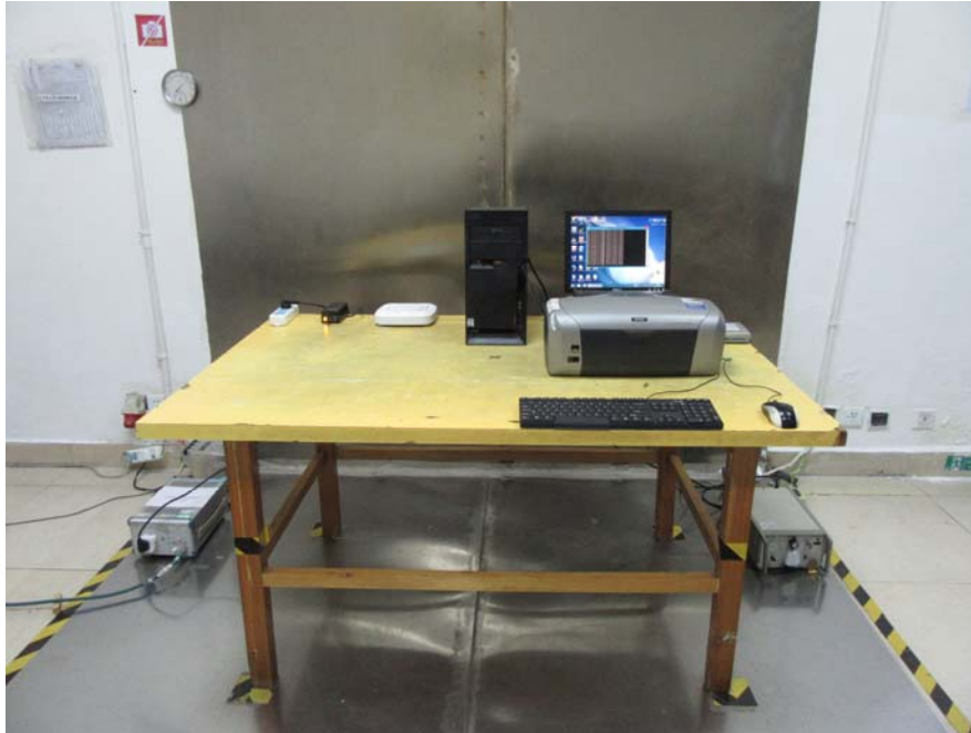
Conducted Emission Front View
