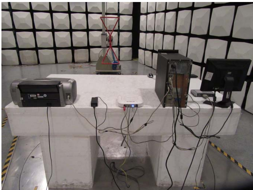
Radiated Emission Rear View (Below 1 GHz)
