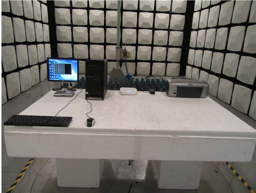
Radiated Emission Front View (Above 1 GHz)
