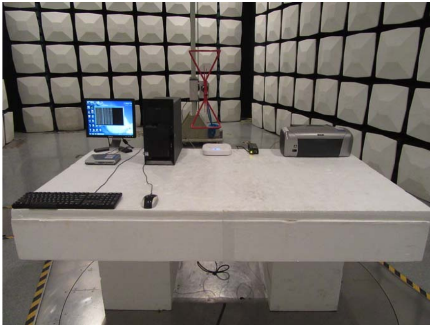
Radiated Emission Front View (Below 1 GHz)
