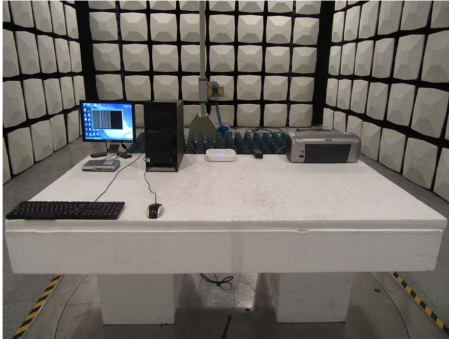
Radiated Emission Front View (Above 1 GHz)
