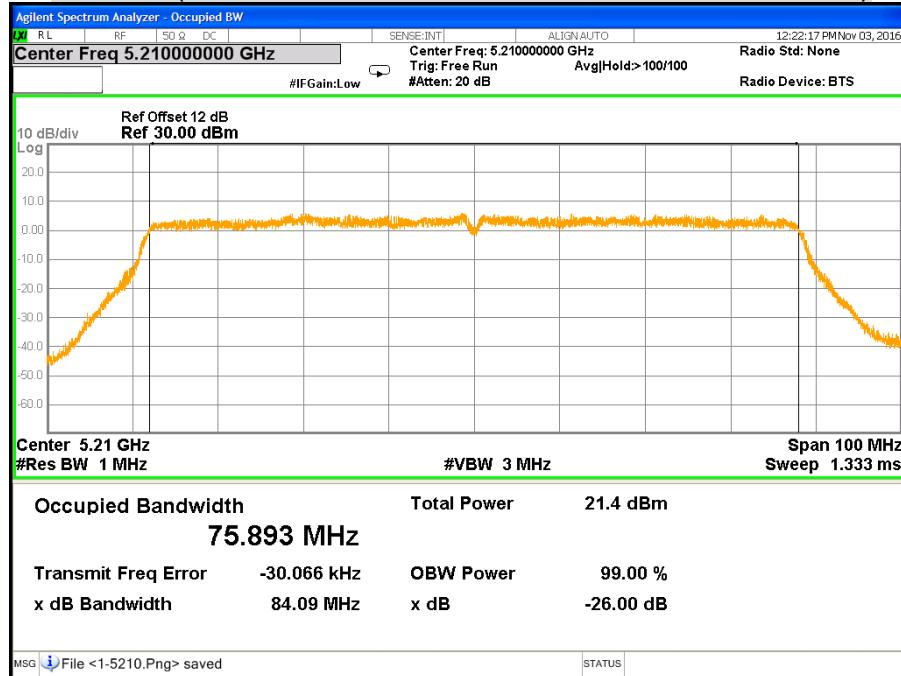
**CH Low (IEEE 802.11ac VHT80 Mode / Band 1 / Chain 2)**
