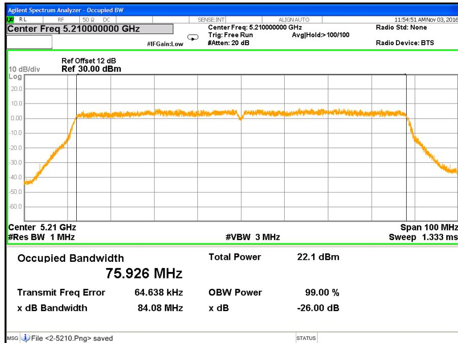
**CH Low (IEEE 802.11ac VHT80 Mode / Band 1 / Chain 3)**
