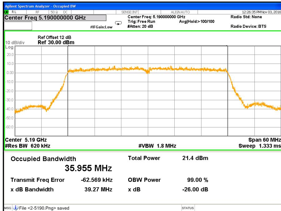
**CH High (IEEE 802.11ac VHT40 Mode / Band 1 / Chain 2)**
