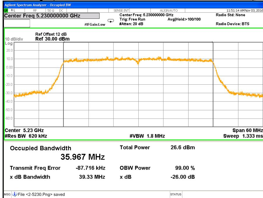
**CH Low (IEEE 802.11ac VHT40 Mode / Band 1 / Chain 3)**
