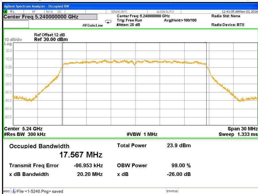
**CH Low (IEEE 802.11ac VHT20 Mode / Band 1 / Chain 2)**
