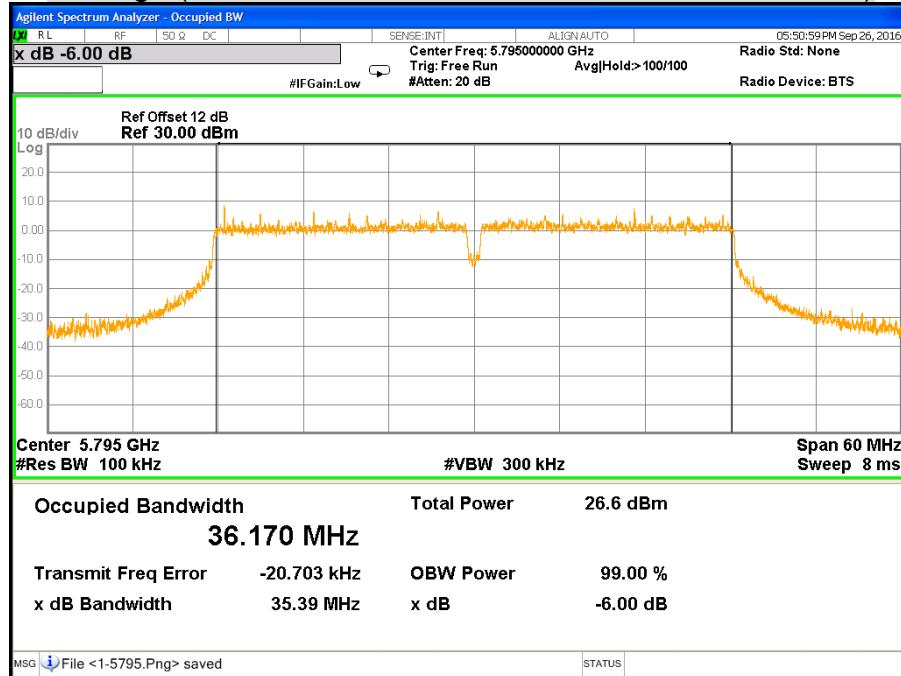
**CH Low (IEEE 802.11ac VHT40 Mode / Band 3 / Chain 2)**
