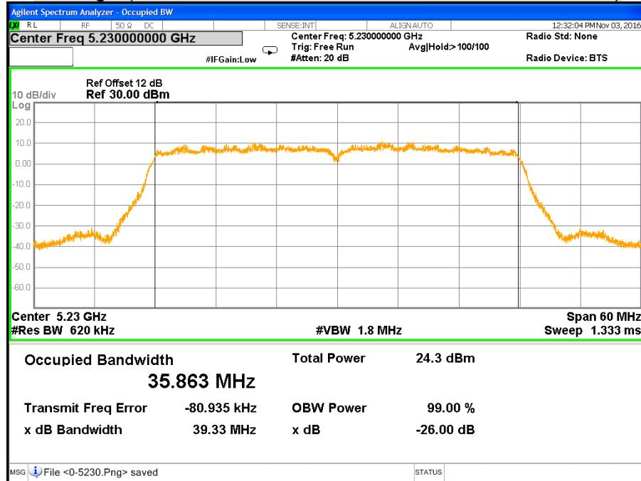
**CH Low (IEEE 802.11ac VHT40 Mode / Band 1 / Chain 1)**
