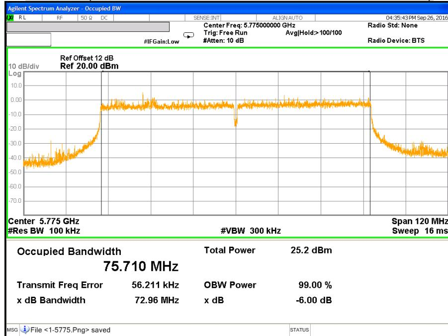
**CH Low (IEEE 802.11ac VHT80 Mode / Band 3 / Chain 2)**
