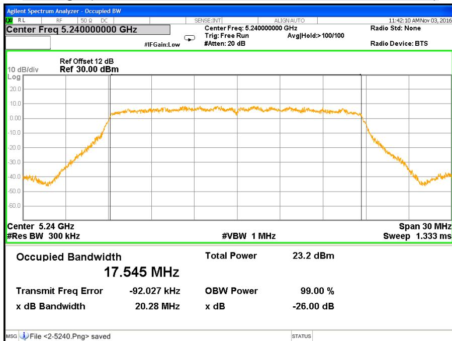
**CH Low (IEEE 802.11ac VHT20 Mode / Band 1 / Chain 3)**
