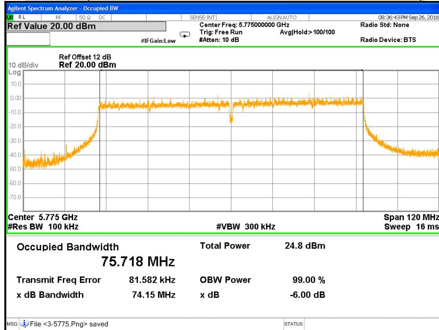
**CH Low (IEEE 802.11ac VHT160 Mode / Band 3 / Chain 0)**
