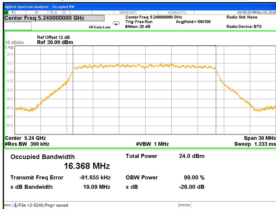
**CH Low (IEEE 802.11a Mode / Band 1 / Chain 3)**
