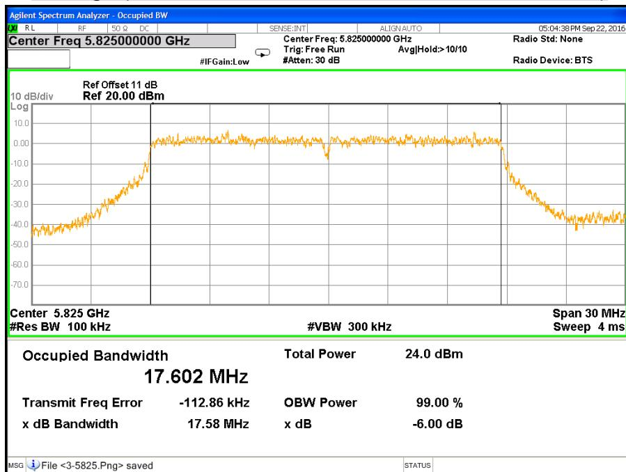
**CH Low (IEEE 802.11ac VHT40 Mode / Band 3 / Chain 0)**
