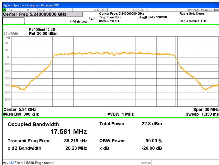
**CH Low (IEEE 802.11ac VHT20 Mode / Band 1 / Chain 2)**
