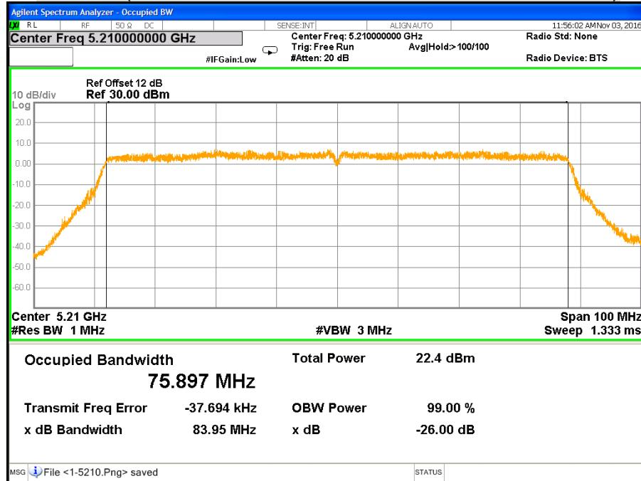
**CH Low (IEEE 802.11ac VHT80 Mode / Band 1 / Chain 2)**
