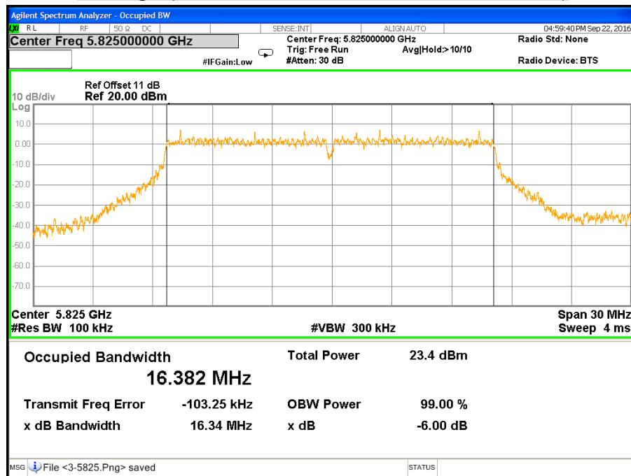
**CH Low (IEEE 802.11ac VHT20 Mode / Band 3 / Chain 0)**
