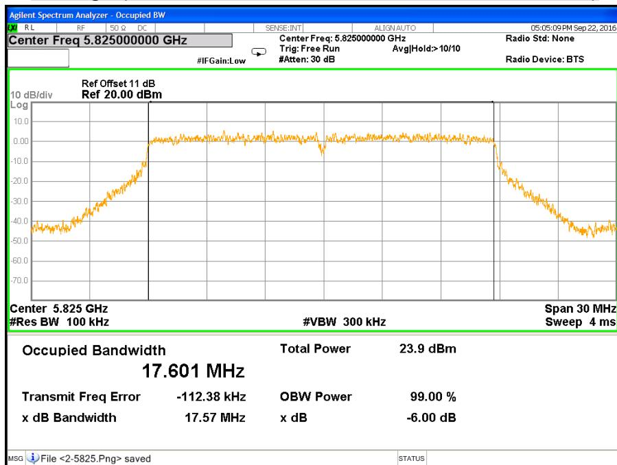
**CH Low (IEEE 802.11ac VHT20 Mode / Band 3 / Chain 3)**
