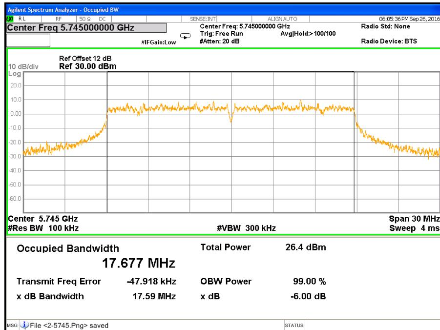
**CH Middle (IEEE 802.11ac VHT20 Mode / Band 3 / Chain 2)**
