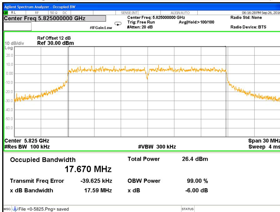
**CH Low (IEEE 802.11ac VHT20 Mode / Band 3 / Chain 1)**
