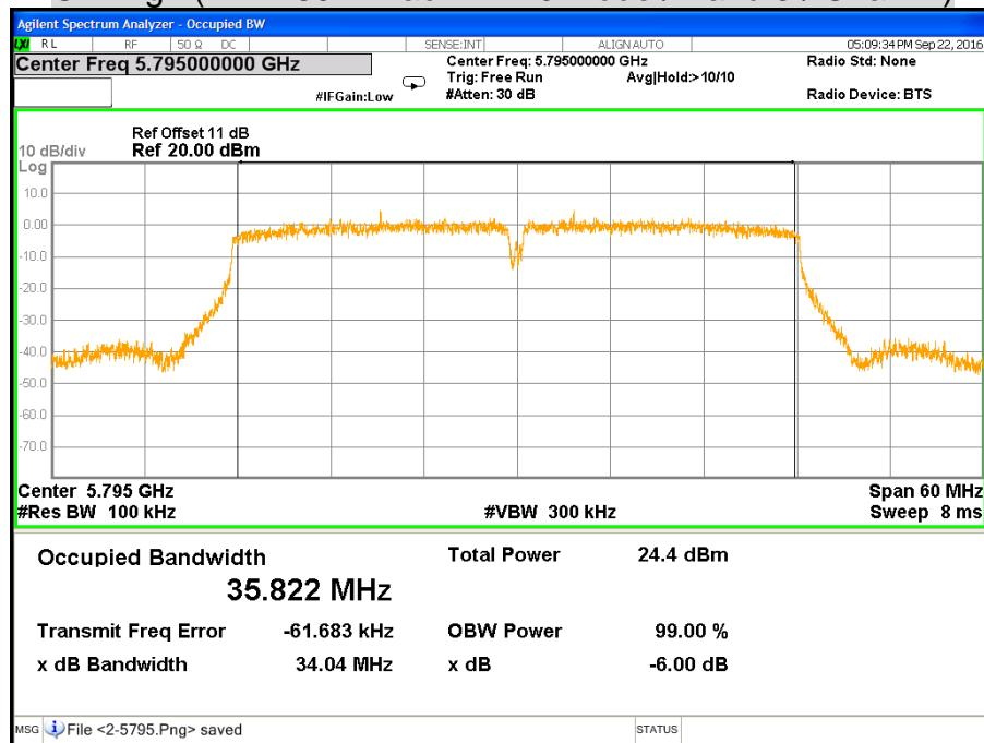
**CH Low (IEEE 802.11ac VHT40 Mode / Band 3 / Chain 3)**
