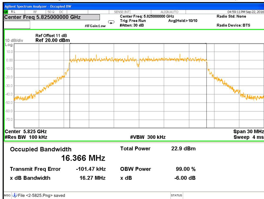
**CH Low (IEEE 802.11a Mode / Band 3 / Chain 3)**
