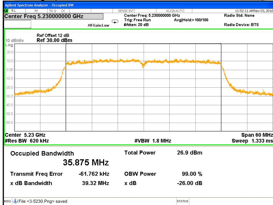
**CH Low (IEEE 802.11ac VHT80 Mode / Band 1 / Chain 0)**
