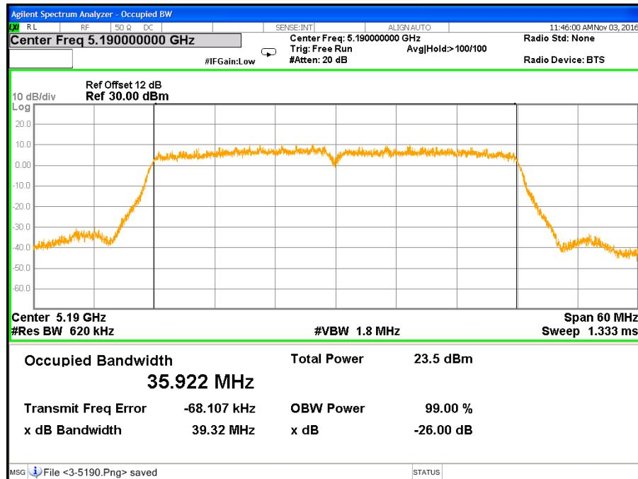
**CH High (IEEE 802.11ac VHT40 Mode / Band 1 / Chain 3)**
