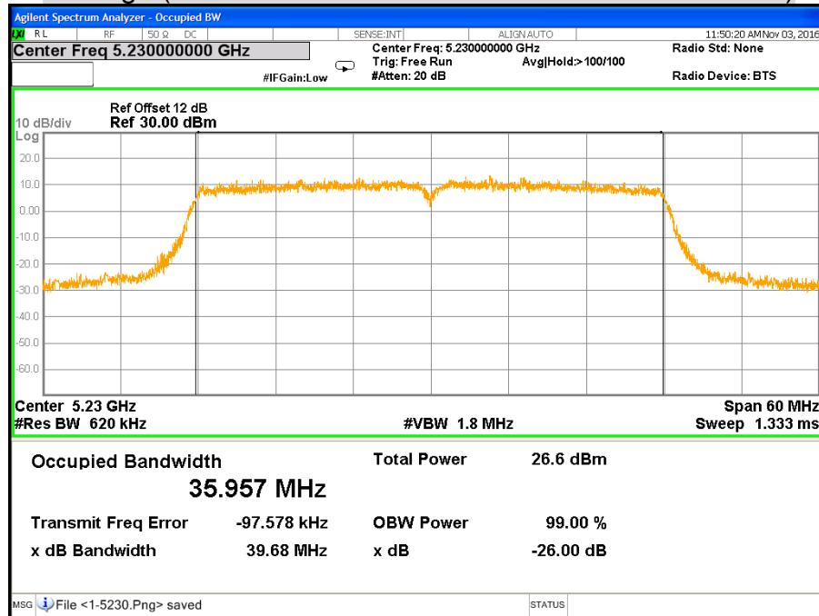
**CH Low (IEEE 802.11ac VHT40 Mode / Band 1 / Chain 2)**
