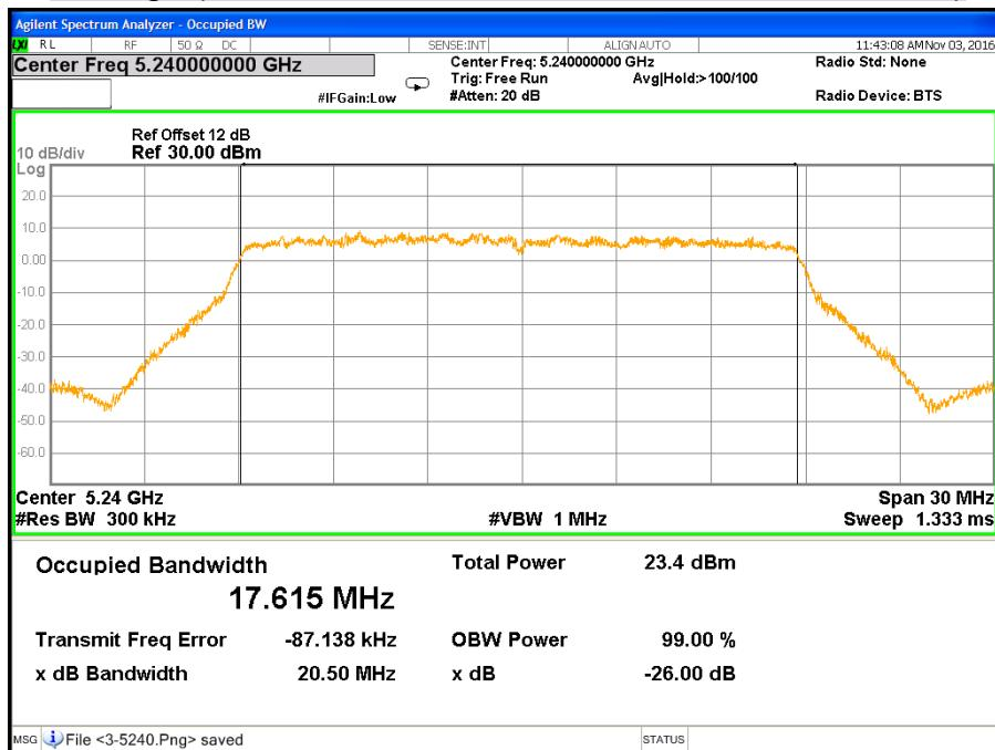
**CH Low (IEEE 802.11ac VHT40 Mode / Band 1 / Chain 0)**
