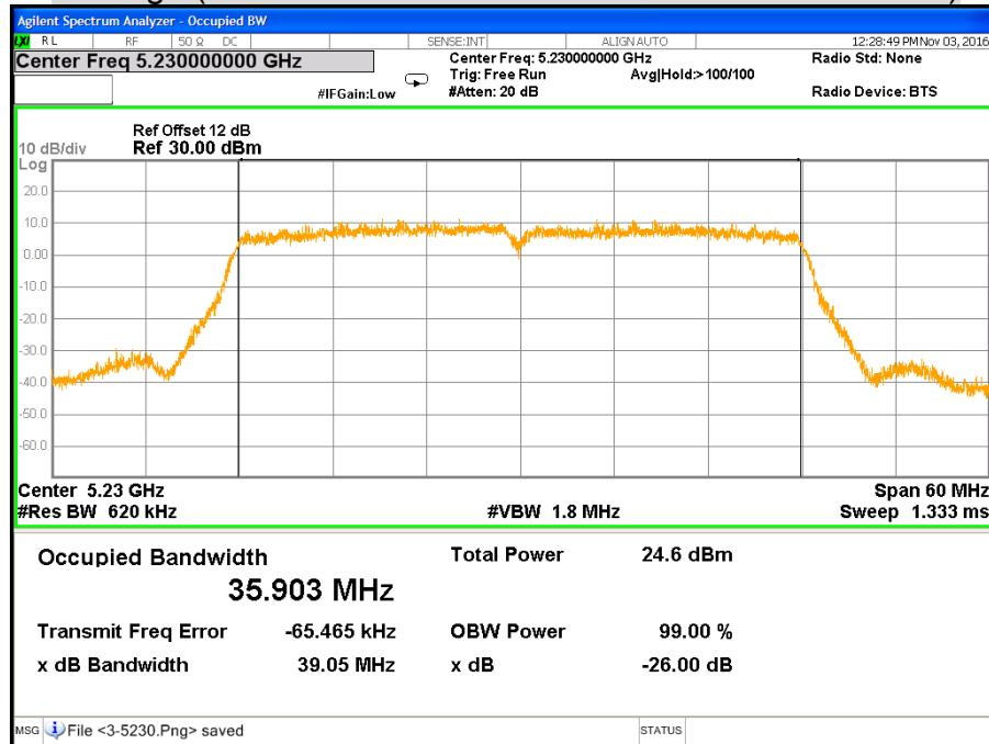
**CH Low (IEEE 802.11ac VHT80 Mode / Band 1 / Chain 0)**
