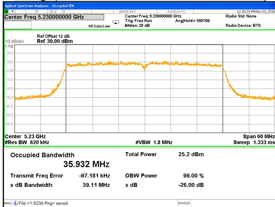
**CH Low (IEEE 802.11ac VHT40 Mode / Band 1 / Chain 2)**
