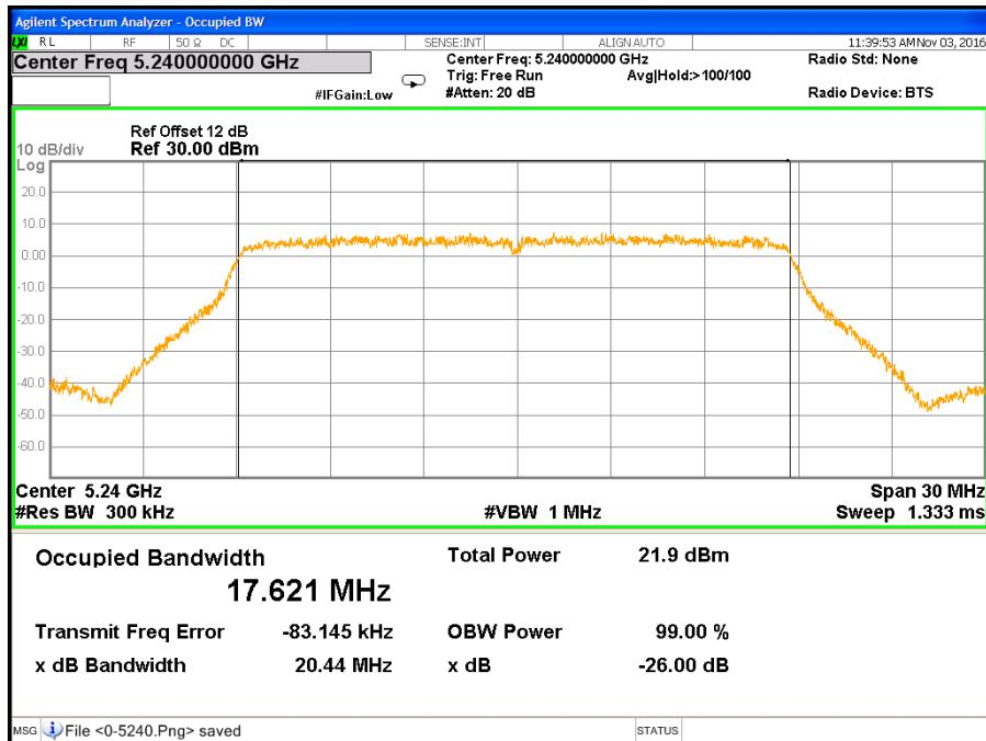
**CH Low (IEEE 802.11ac VHT20 Mode / Band 1 / Chain 1)**
