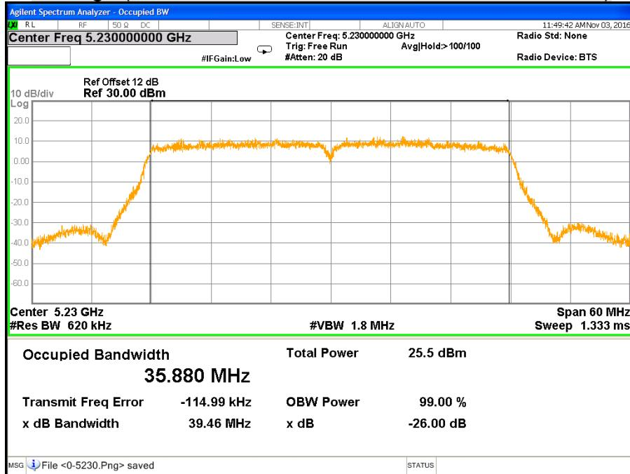
**CH Low (IEEE 802.11ac VHT40 Mode / Band 1 / Chain 1)**
