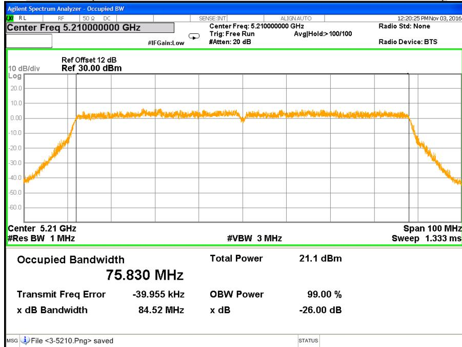
**CH Low (IEEE 802.11ac VHT160 Mode / Band 1 / Chain 0)**
