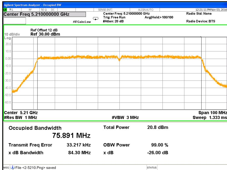
**CH Low (IEEE 802.11ac VHT80 Mode / Band 1 / Chain 3)**
