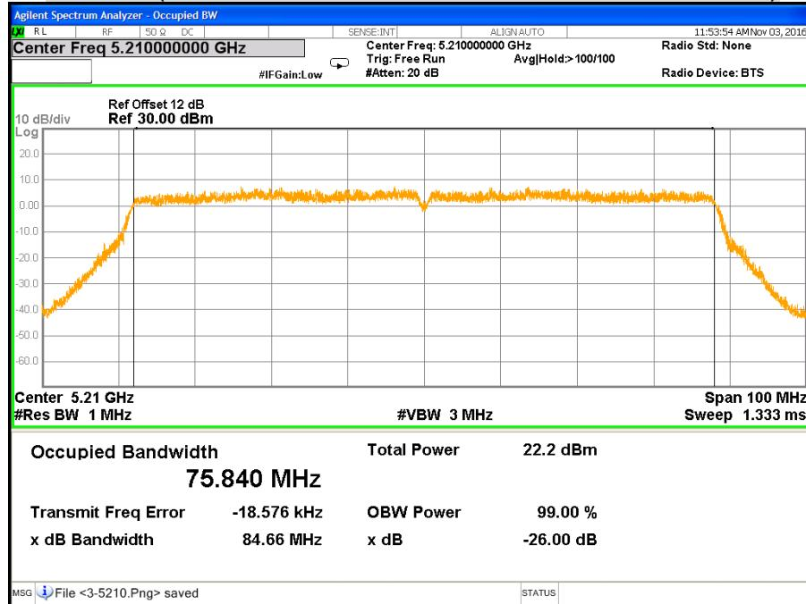
**CH Low (IEEE 802.11ac VHT160 Mode / Band 1 / Chain 0)**
