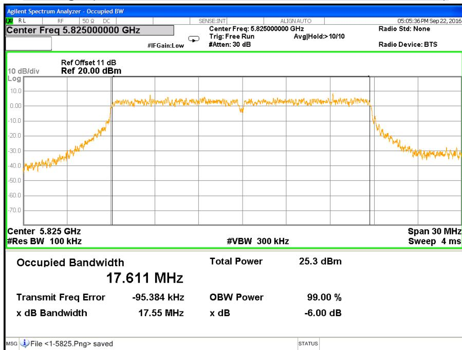
**CH Low (IEEE 802.11ac VHT20 Mode / Band 3 / Chain 2)**
