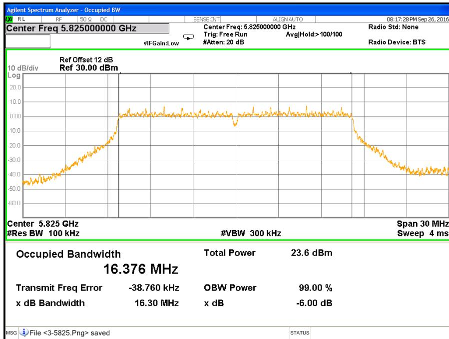
**CH Low (IEEE 802.11ac VHT20 Mode / Band 3 / Chain 0)**
