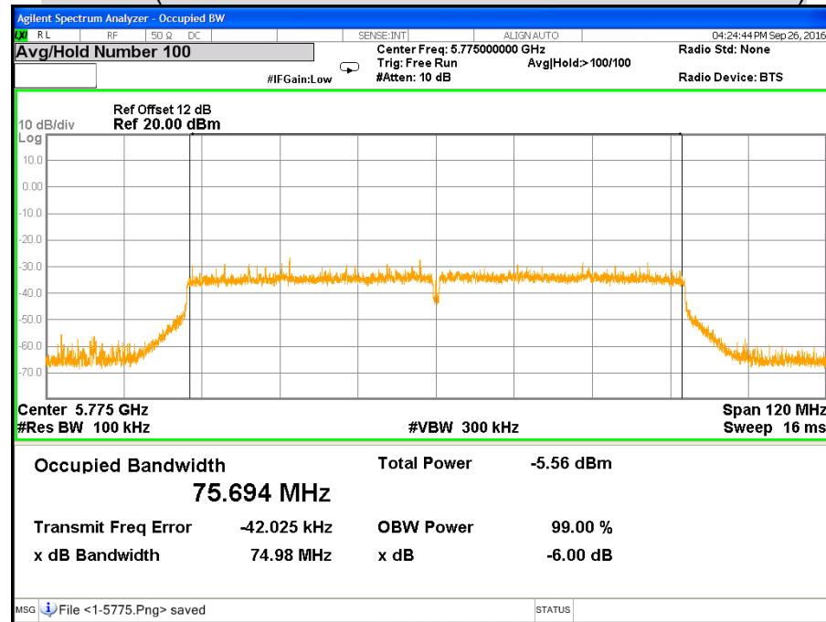
**CH Low (IEEE 802.11ac VHT160 Mode / Band 3 / Chain 2)**
