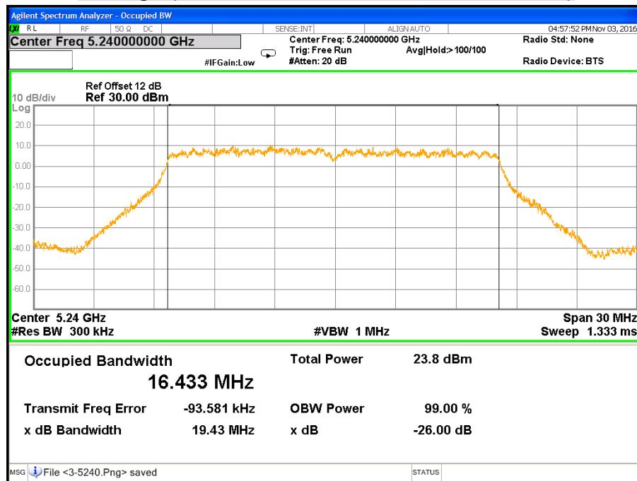
**CH Low (IEEE 802.11ac VHT20 Mode / Band 1 / Chain 0)**
