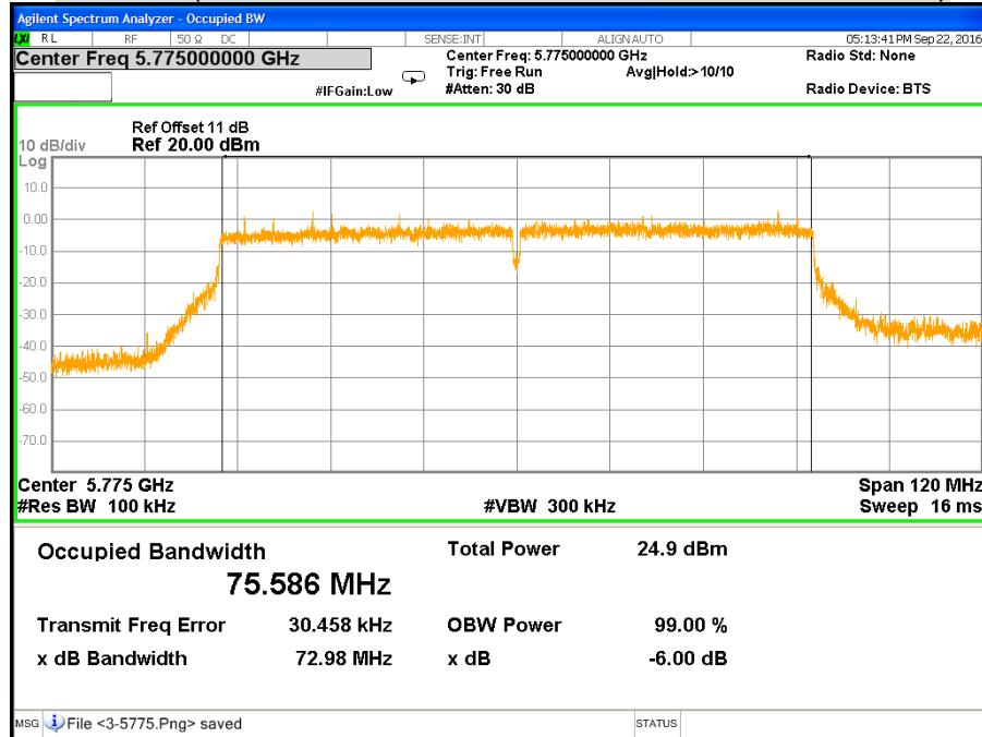
**CH Low (IEEE 802.11ac VHT160 Mode / Band 3 / Chain 0)**
