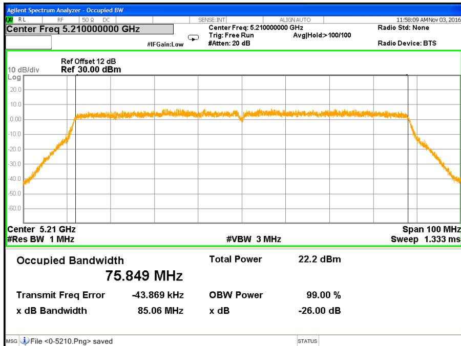
**CH Low (IEEE 802.11ac VHT160 Mode / Band 1 / Chain 1)**
