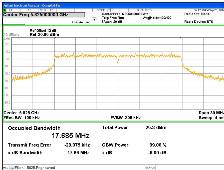
**CH Low (IEEE 802.11ac VHT20 Mode / Band 3 / Chain 2)**
