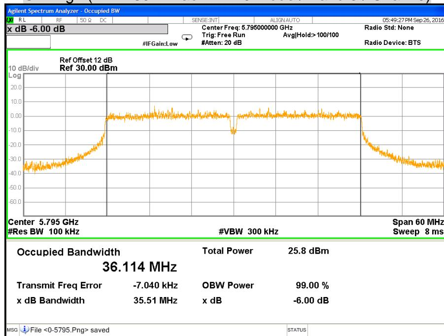
**CH Low (IEEE 802.11ac VHT40 Mode / Band 3 / Chain 1)**
