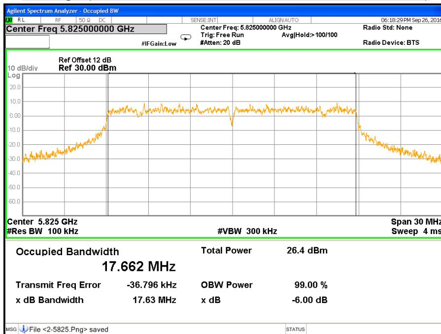
**CH Low (IEEE 802.11ac VHT20 Mode / Band 3 / Chain 3)**
