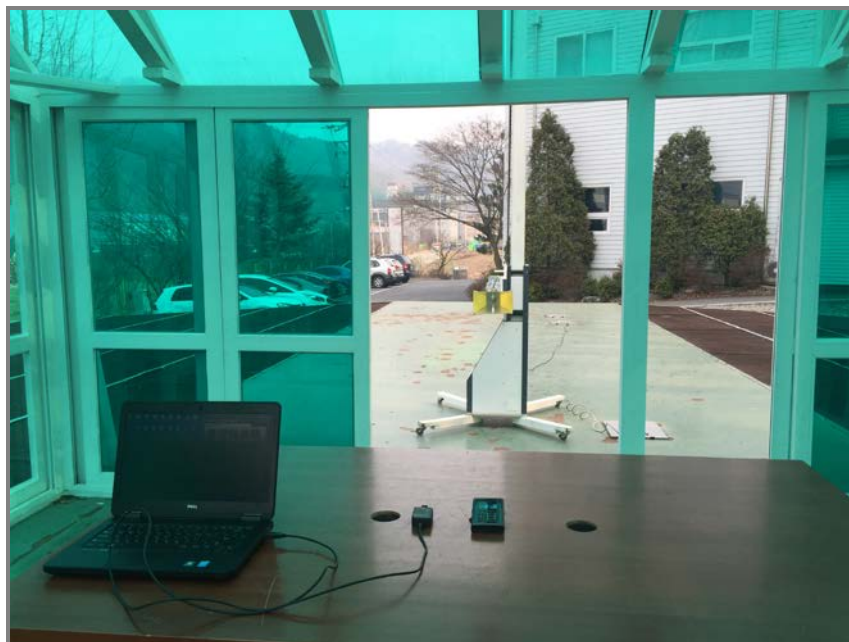
Photo of radiated spurious emission at above 1 000MHz (BLE mode)
