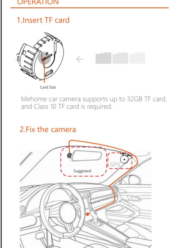
2.2 Connect the USB power cable with camera and car charger, hiding the cable like the sketch map above.
