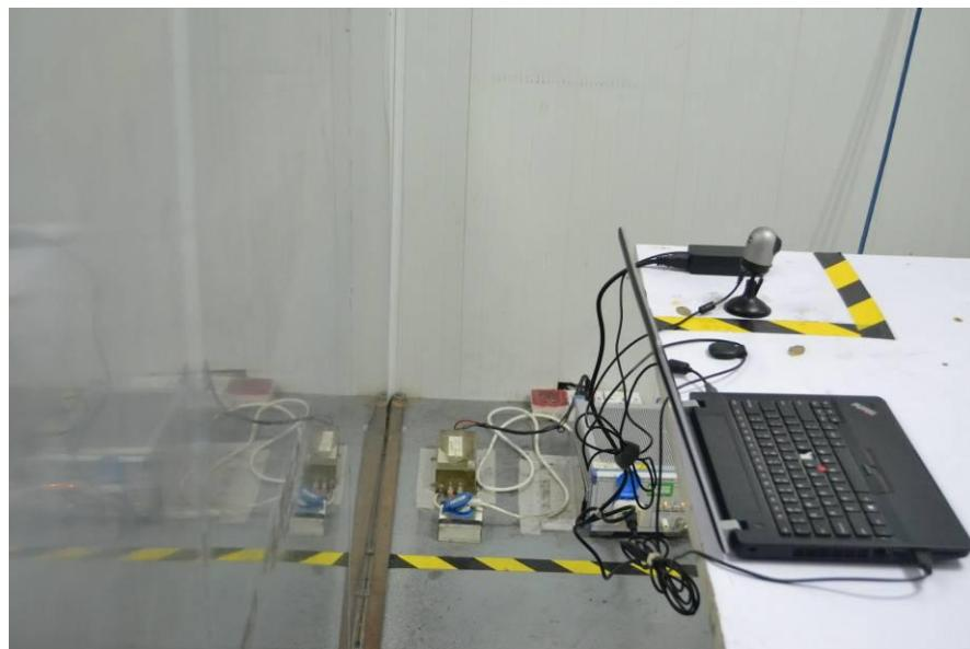
**RADIATED EMISSION TEST****Below 1GHz**
