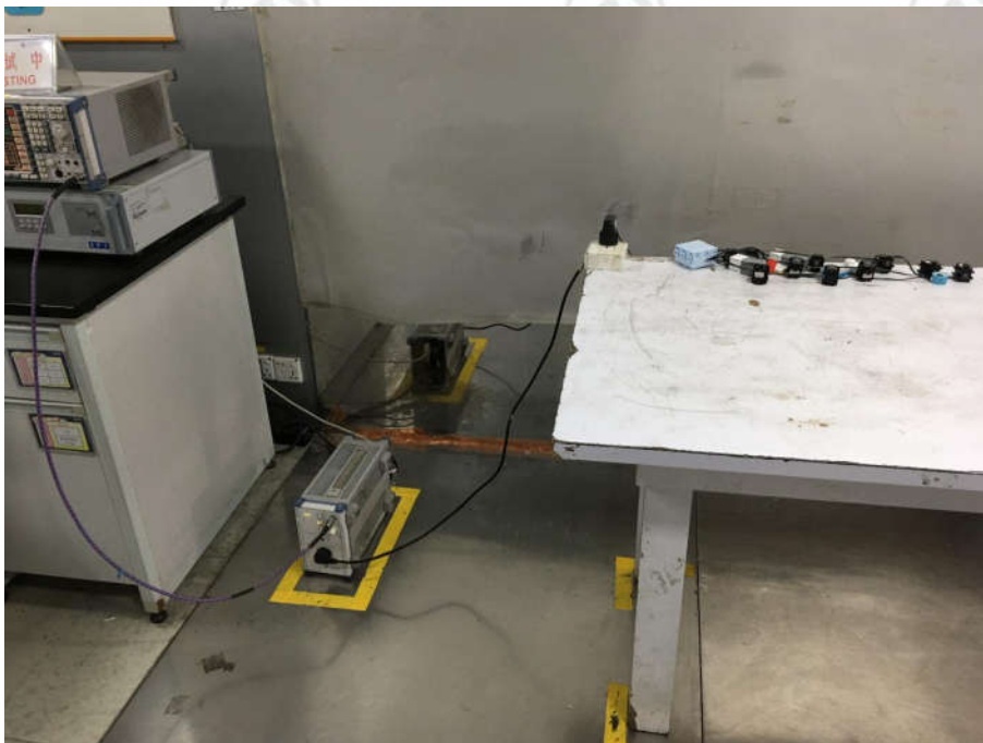
Conducted Emissions Test Setup
