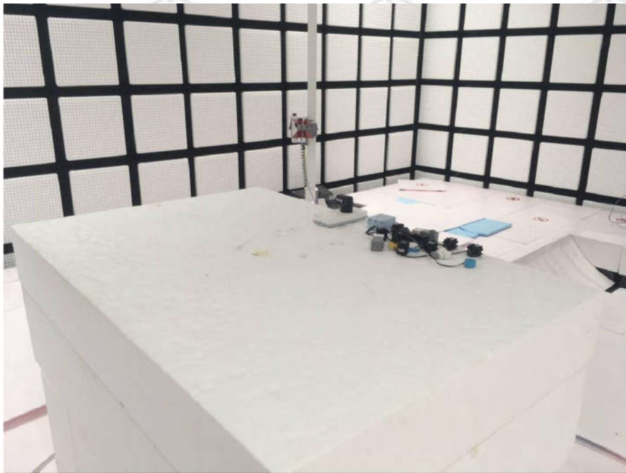
Radiated spurious emission Test Setup-3(Above 1GHz)
