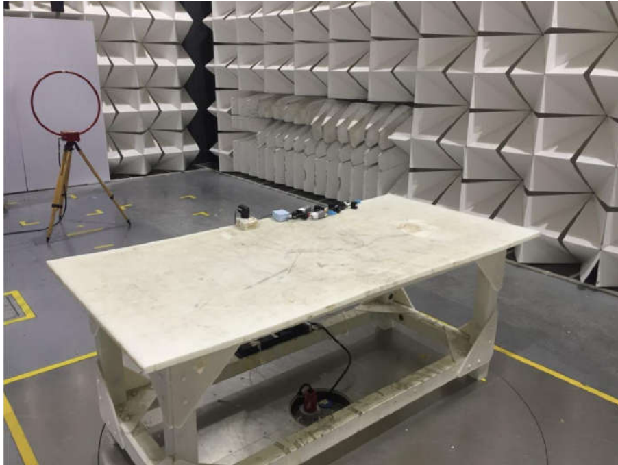
Radiated spurious emission Test Setup-1(Below 30MHz)
