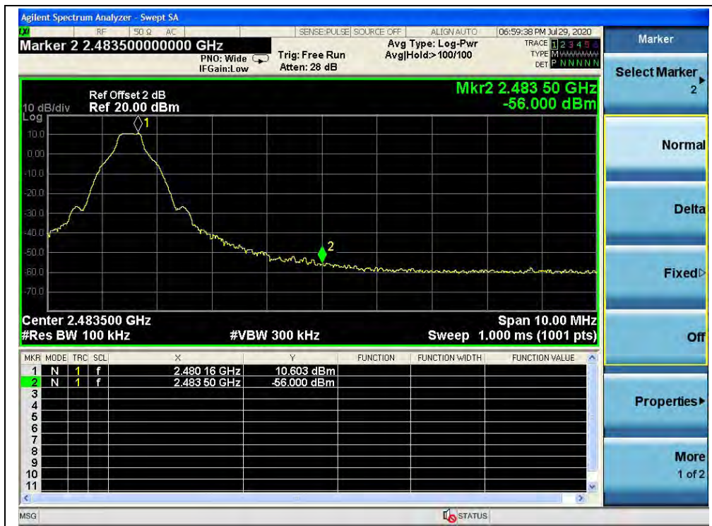
(Band edge, Channel 78, GFSK)
