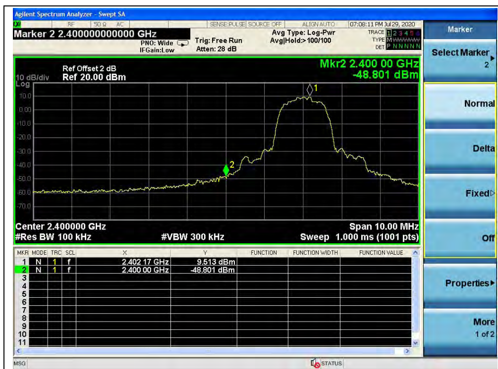
(Band edge, Channel 0, 8-DPSK)
