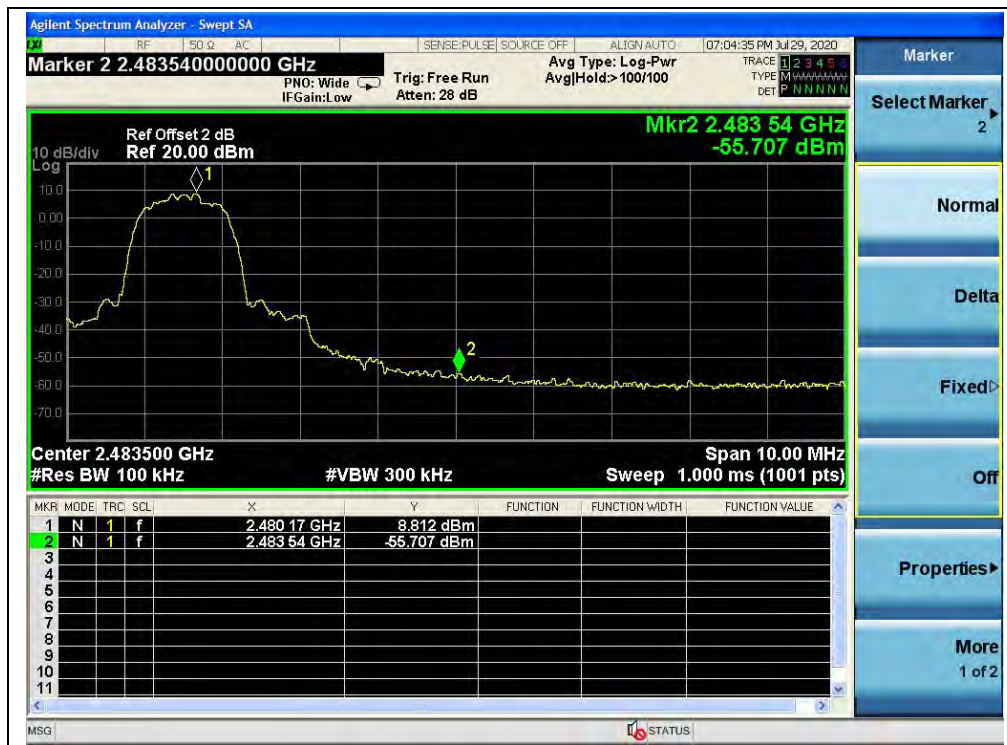
(Band edge, Channel 78, 8-DPSK)
