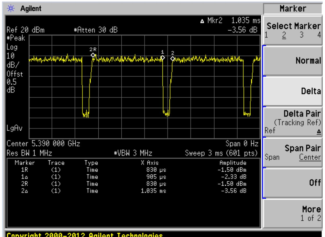
The channel loading Specification of Ton/ (Ton +Toff) as the file streaming between master to client is 87.4%.
