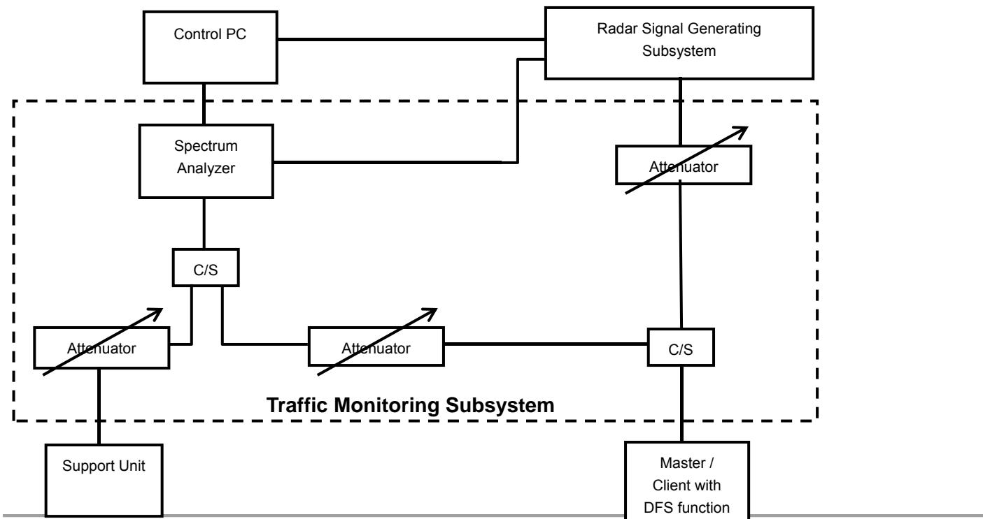
The test transmission will always be from the Master Device to the Client Device. While the Client device is set up to associate with the Master device and play the MPEG file (6  $\frac{1}{2}$  Magic Hours) from Master device, the designated MPEG test file and instructions are located at: <http://ntiacsd.ntia.doc.gov/dfs/>.
