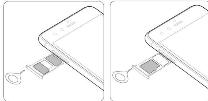
SIM SLOT 1: Nano-SIM card slot
