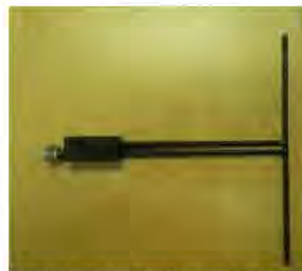
Figure 1 – MVG COMOSAR Validation Dipole
