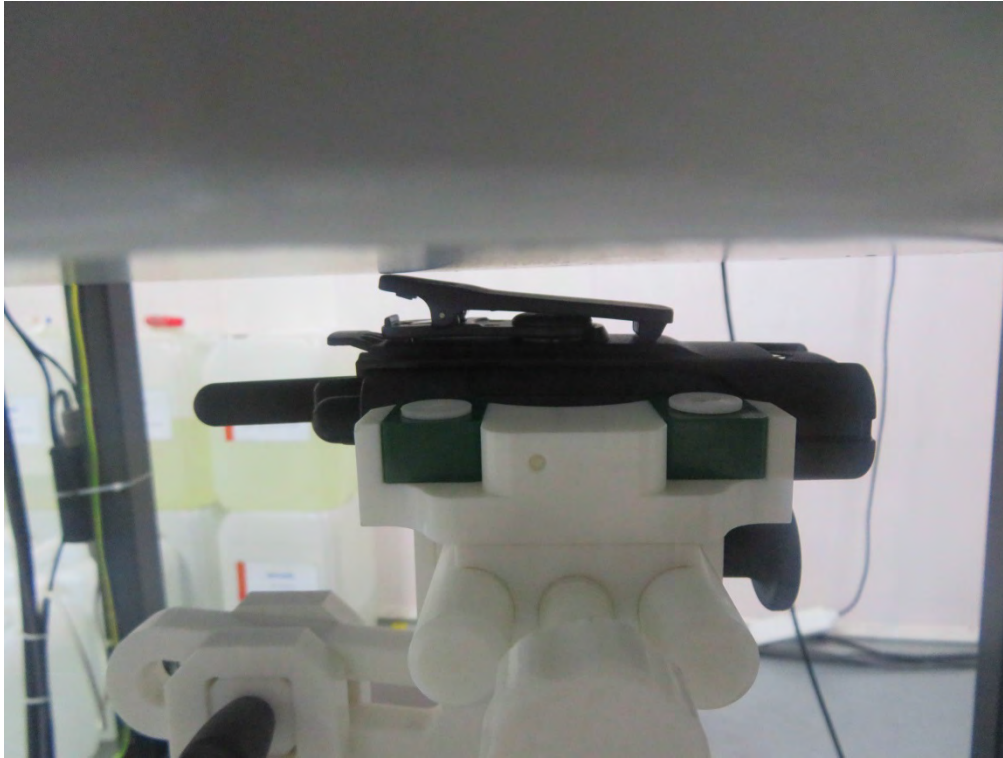
0mm body-worn Side Setup Photo
