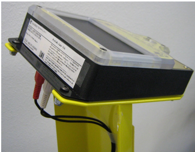
Closer View of the ESD Tester box (Same Unit is used on both Agent and Deputy Agent models) - Back & Left View -
