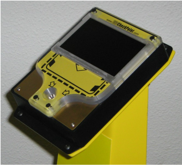
Closer View of the ESD Tester box (Same Unit is used on both Agent and Deputy Agent models) - Top, Right & Front View -
