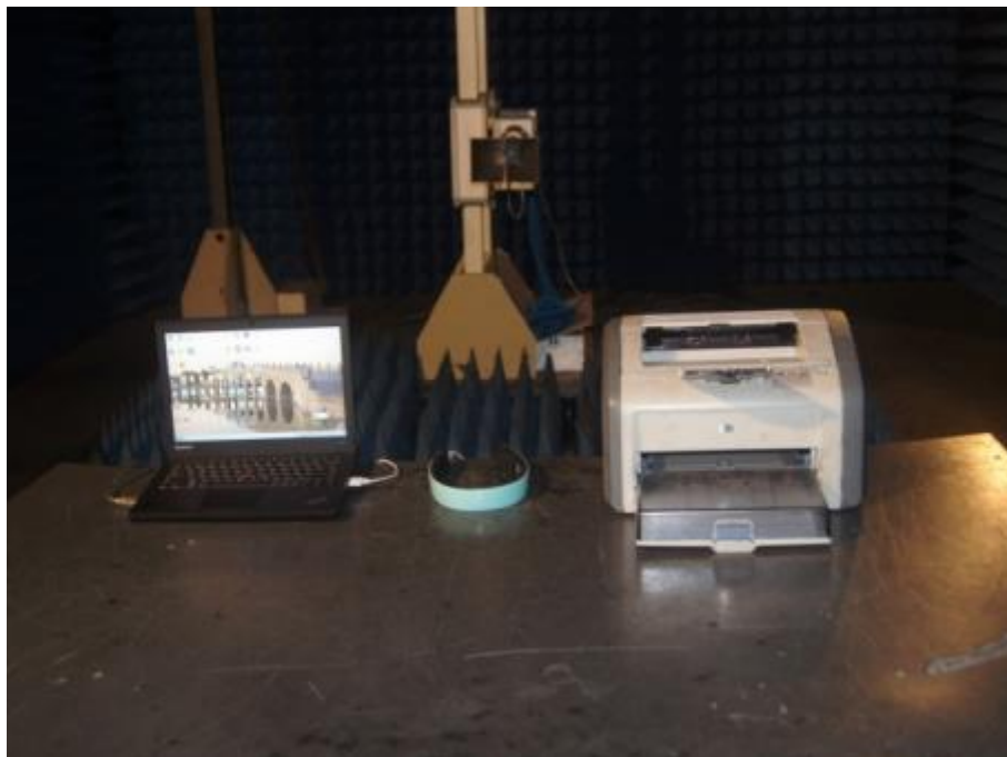
Photograph 8: Set-up for Radiated Emission (1GHz ~ 6GHz)
