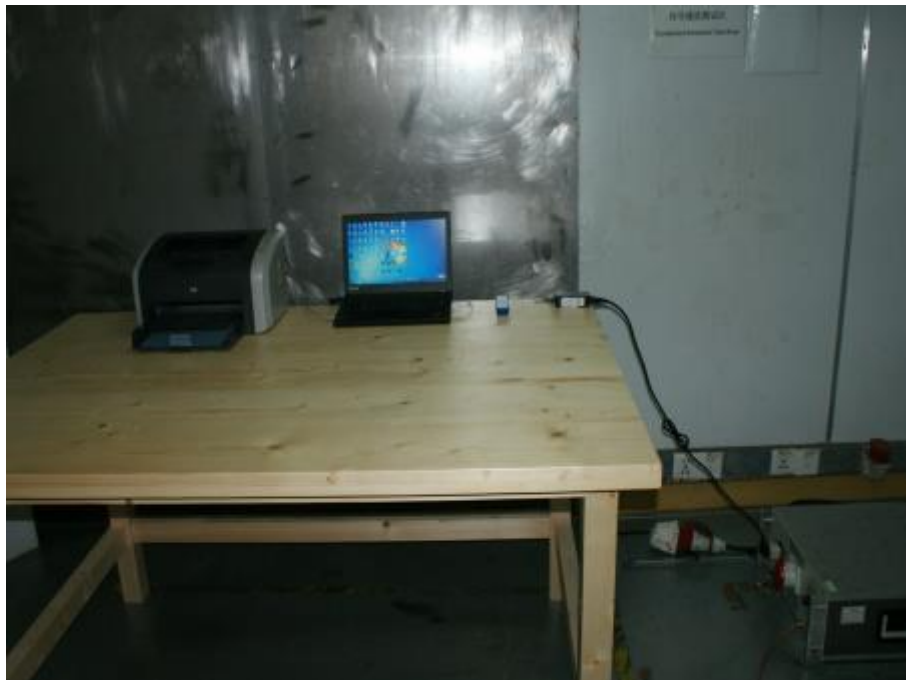
Photograph 6: Set-up for Conducted Emission
