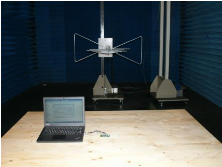
Photograph 4: Set-up for Radiated Spurious Emission (1GHz ~ 18GHz)
