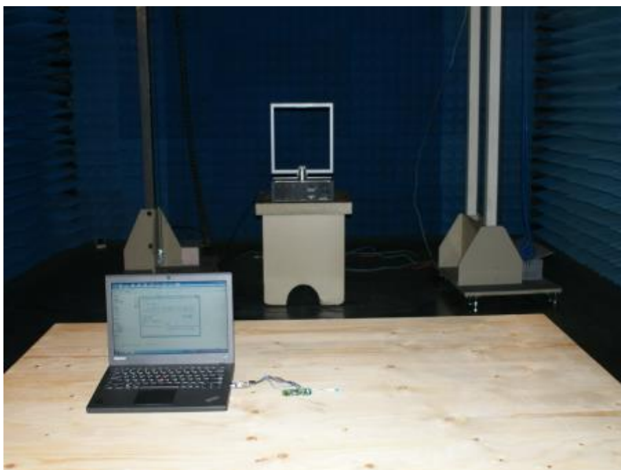
Photograph 2: Set-up for Radiated Spurious Emission (9kHz ~ 30MHz)
