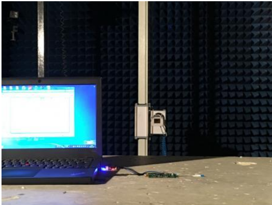
Photograph 6: Set-up for Conducted Emission
