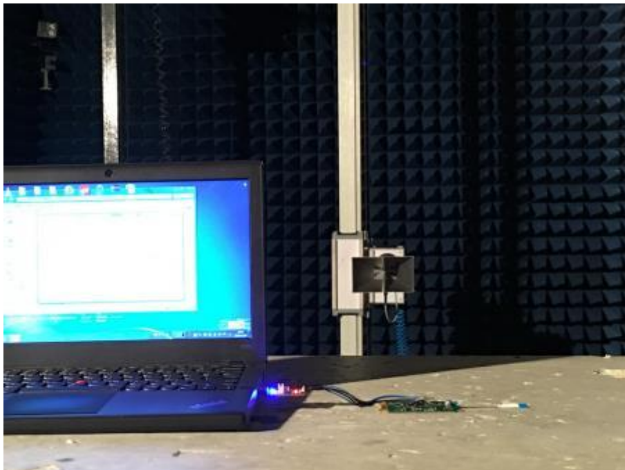
Photograph 4: Set-up for Radiated Spurious Emission (1GHz ~ 18GHz)
