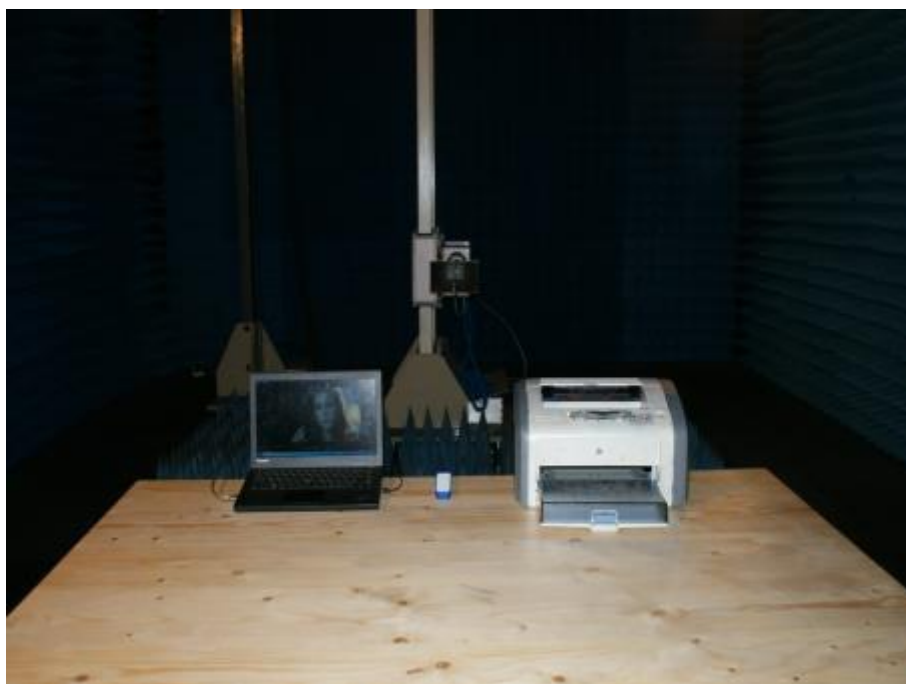
Photograph 8: Set-up for Radiated Emission (1GHz ~ 6GHz)
