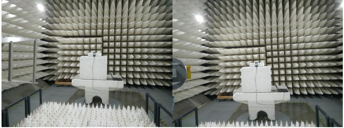
Photograph No.4 Spurious and band edge emissions measurement setup in the anechoic chamber above 1 GHz
