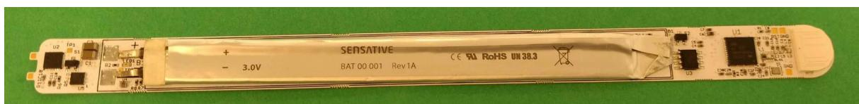
Radio part including transceiver and antenna
