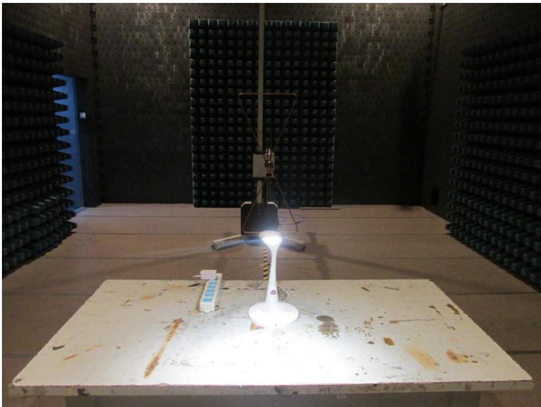
Radiated Emission Test setup photos
