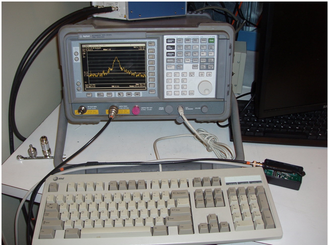
Photo 7.4-1 – Bandwidth and Time Domain Test Set-up
