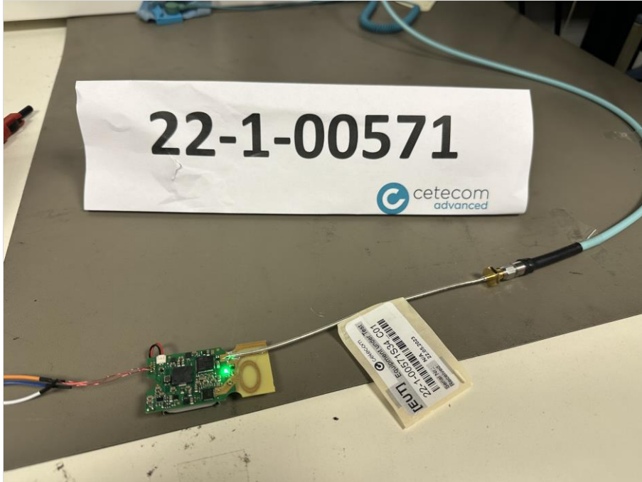
Photograph 1: EUT setup conducted measurement, close up view
