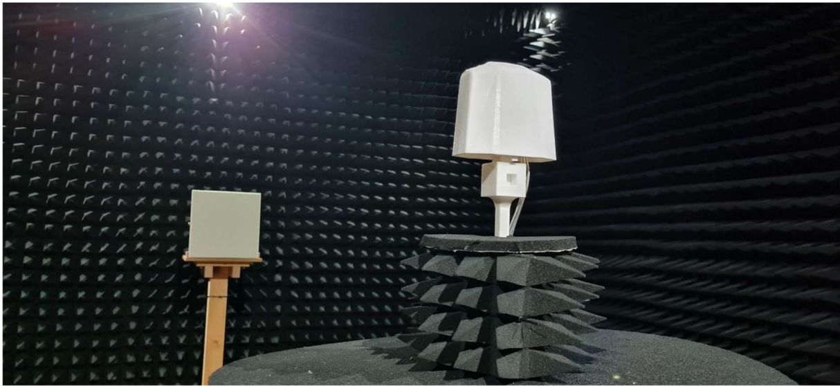
figure 12 - measurement setup for horizontal diagram measurement
