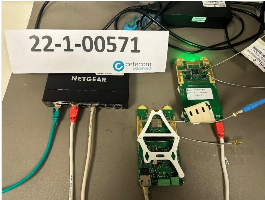
Photograph 1: EUT setup conducted measurement, close up view
