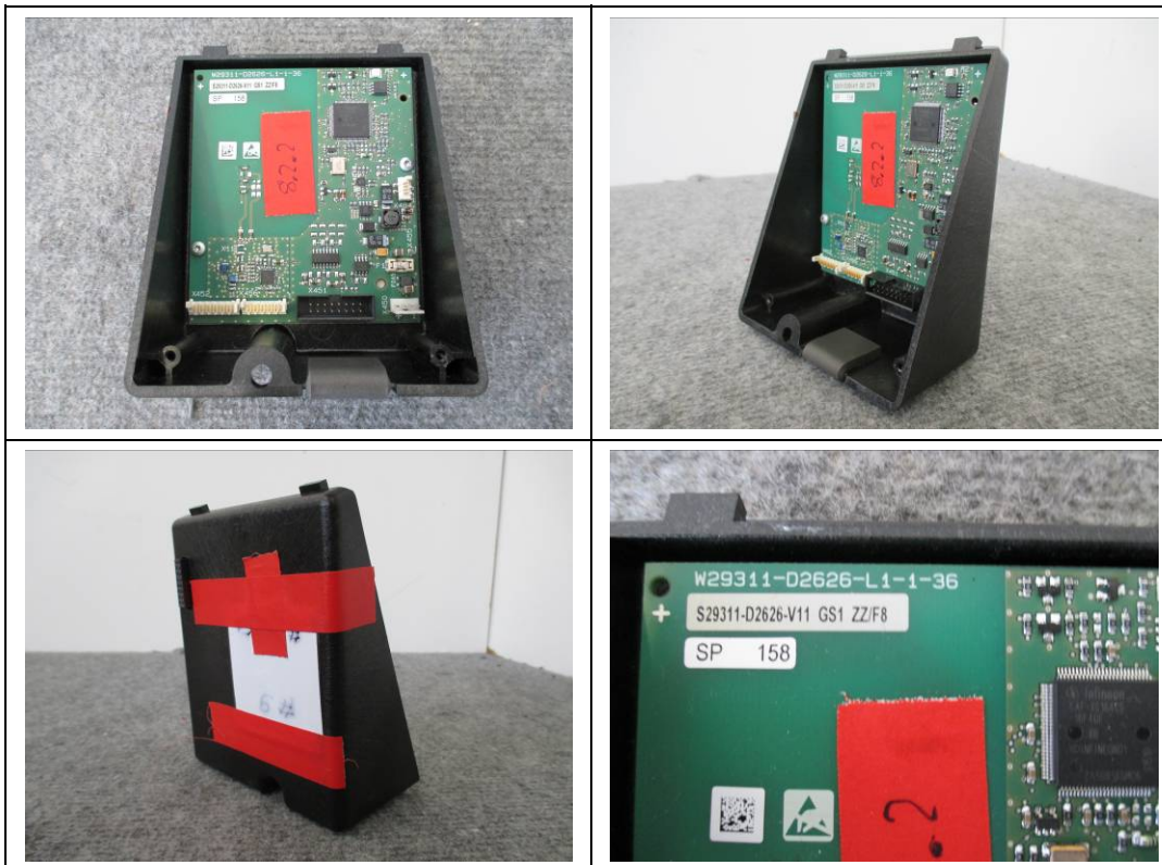
Figure 7-10: S29311-D2626-V11 with antenna on board
