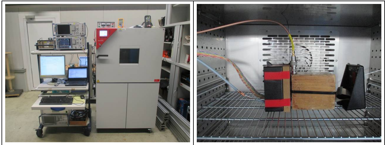
Figure 7-9: Test Setup – Frequency Stability with voltage or Temperature variation
