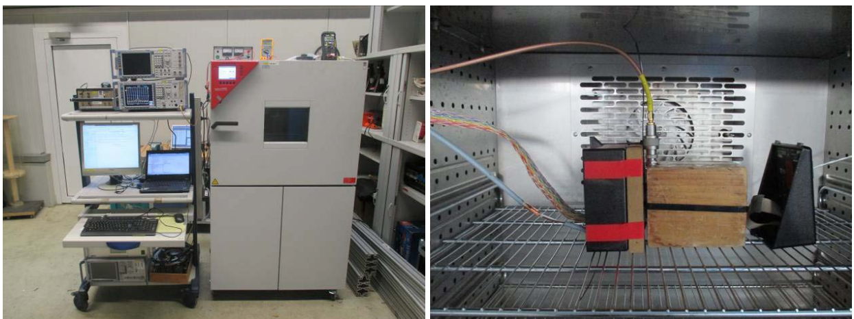
Figure 4: test setup for frequency stability
