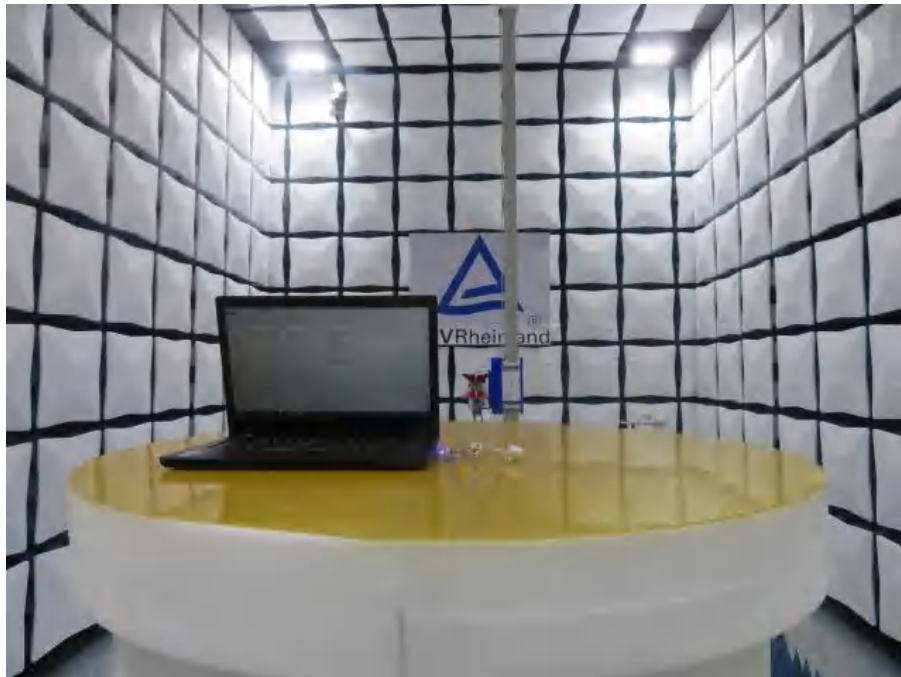
Photograph 2: Set-up for Radiated Spurious Emission, Above 1GHz
