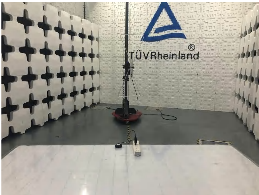
Photograph 4: Set-up for Radiated Emission, Below 1GHz
