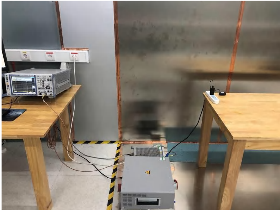
Photograph 3: Set-up for Conducted Emission on AC Mains
