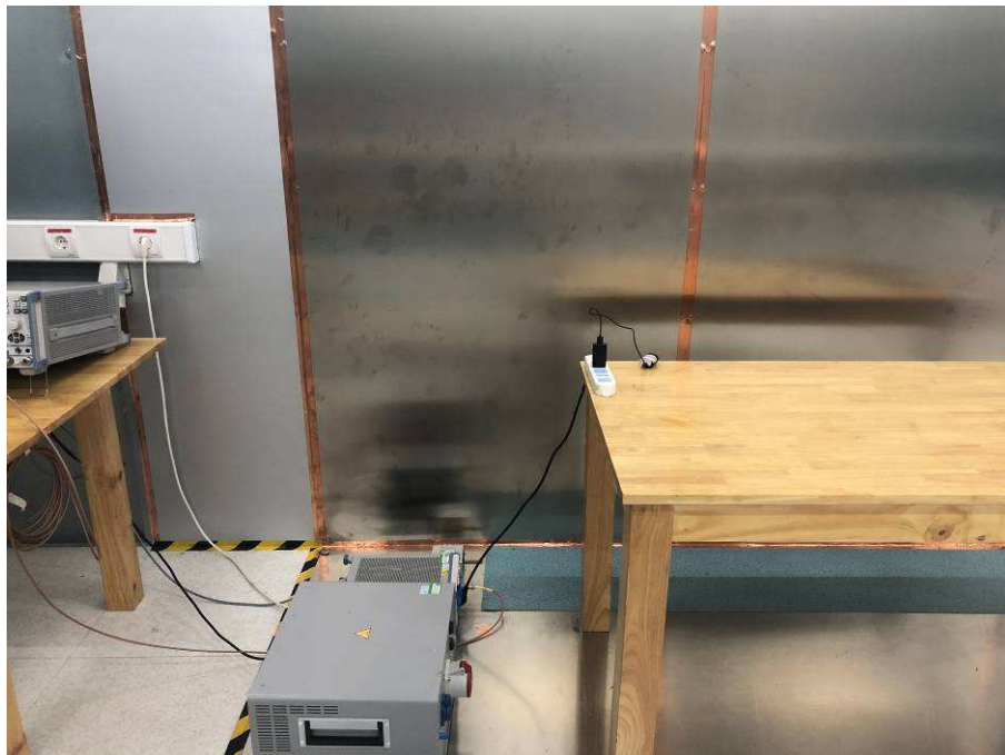
Photograph 3: Set-up for Conducted Emission on AC Mains
