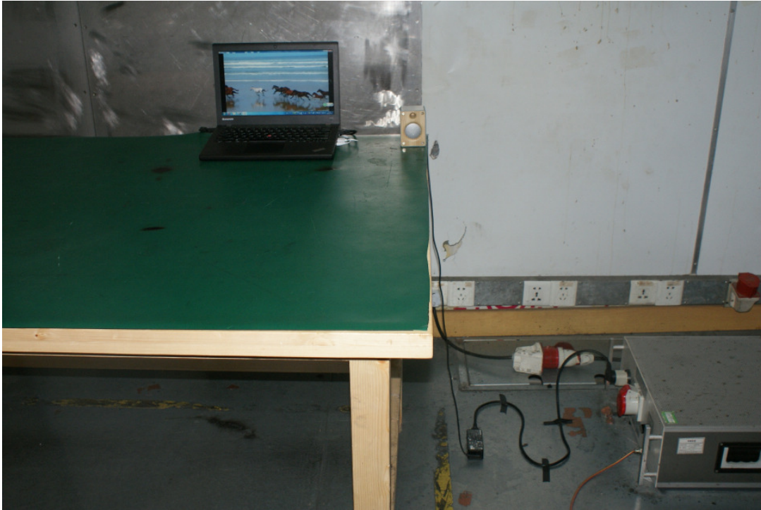
Photograph 6: Set-up for Radiated Emissions, below 1GHz
